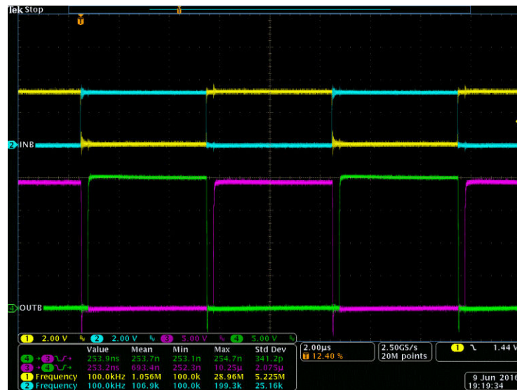
Figure 8-5. Bench Test Waveform for INA/B and OUTA/B
