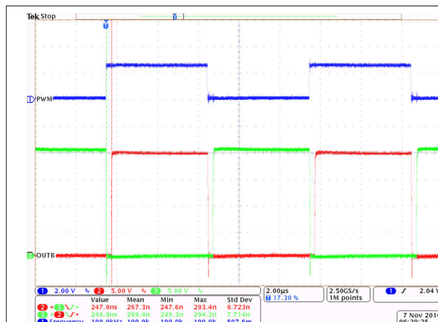
Figure 9-5. Bench Test Waveform for PWM and OUTA/B
