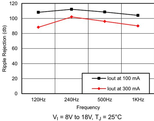
Figure 5-9. PSRR vs Frequency and I<sub>O</sub> (Legacy Chip)
