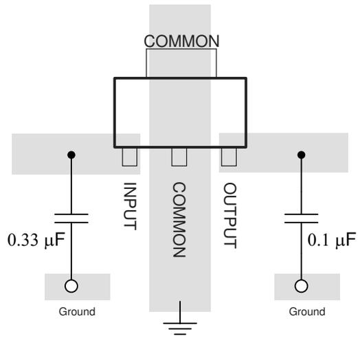
Figure 7-12. Layout Diagram
