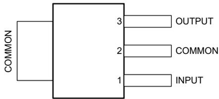
**Figure 4-1. DCY Package, 3-Pin SOT-223 (Top View)**
