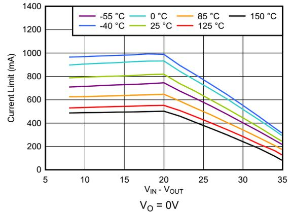
**Figure 5-6.  $I_{CL}$  vs Input Voltage (New Chip)**
