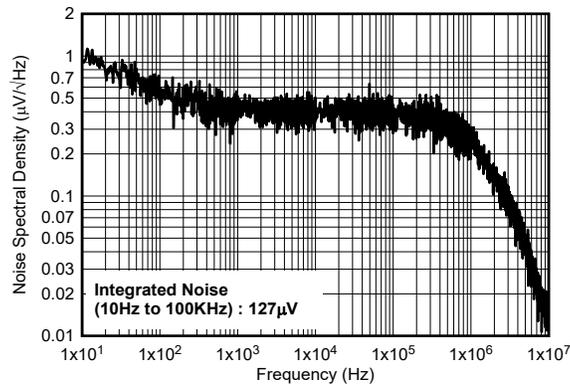
V<sub>IN</sub> = 10V, V<sub>OUT</sub> = 5V, I<sub>OUT</sub> = 100mA, C<sub>OUT</sub> = 0.1µF
