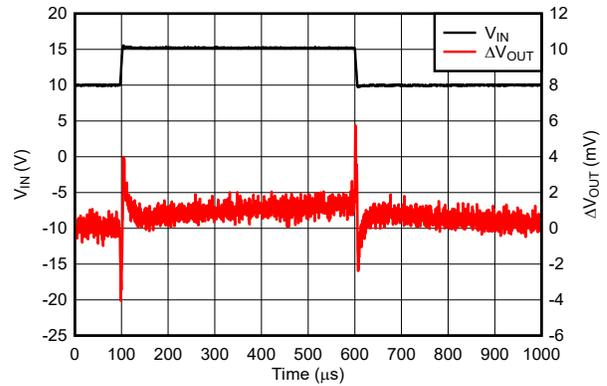
$V_O = 5\text{V}$ ,  $dV_{IN}/dt = 1\text{V}/\mu\text{s}$ ,  $I_{OUT} = 350\text{mA}$ ,  $C_{OUT} = 0.1\mu\text{F}$
