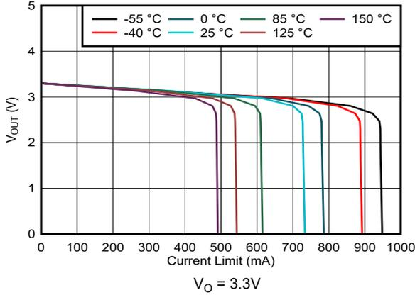
Figure 5-7. Output Voltage vs I<sub>CL</sub> (New Chip)
