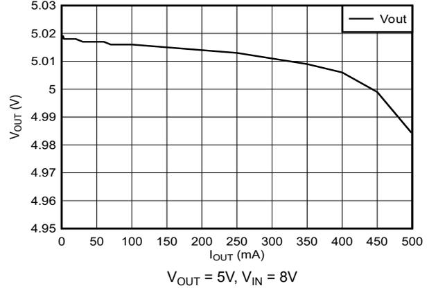
**Figure 5-2. Load Regulation at  $T_J = 25^\circ\text{C}$  (New Chip)**
