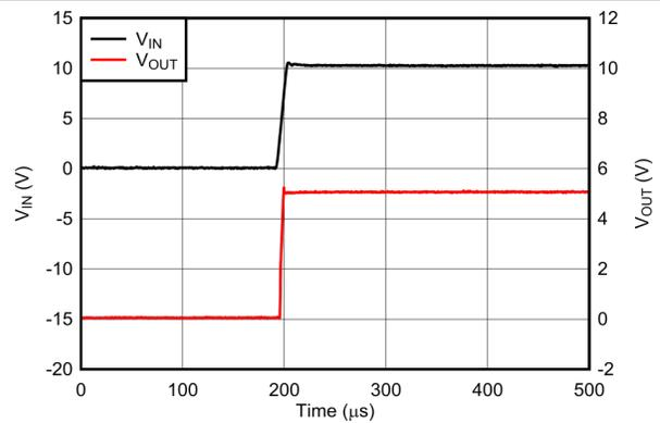
$V_{IN} = 0\text{V}$  to  $10\text{V}$ ,  $V_{OUT} = 5\text{V}$ ,  $I_{OUT} = 100\text{mA}$ ,  $dV_{IN}/dt = 1\text{V}/\mu\text{s}$ ,  $C_{OUT} = 0.1\mu\text{F}$
