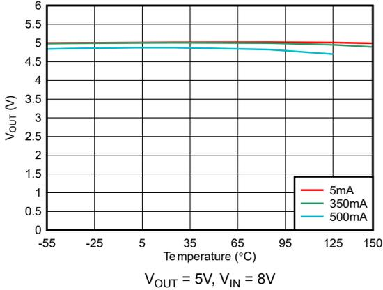
**Figure 5-1. Output Voltage vs Temperature (New Chip)**
