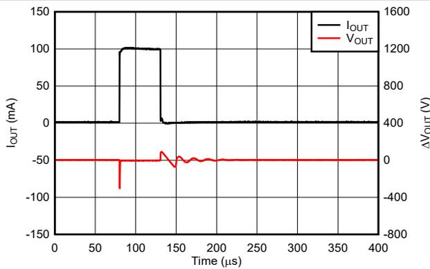
$V_{IN} = 10\text{V}$ ,  $V_{OUT} = 5\text{V}$ ,  $I_{OUT} = 1\text{mA}$  to  $100\text{mA}$ ,  $dI/dt = 1\text{A}/\mu\text{s}$ ,  $C_{OUT} = 0.1\mu\text{F}$
