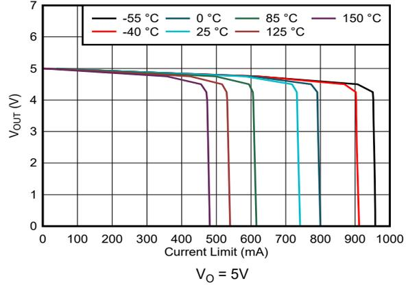
Figure 5-8. Output Voltage vs I<sub>CL</sub> (New Chip)
