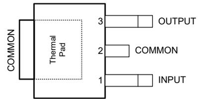
**Figure 4-2. KVU Package, 3-Pin TO-252 (Top View)**
