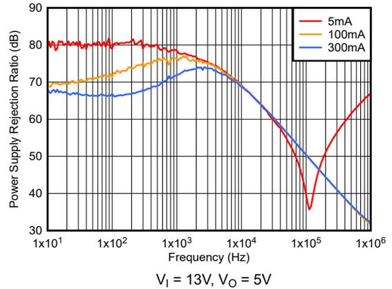
Figure 5-10. PSRR vs Frequency and I<sub>O</sub> (New Chip)
