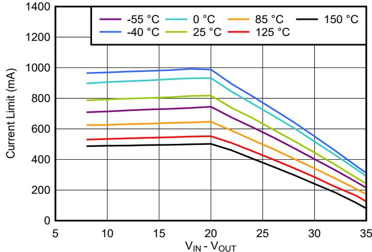
**Figure 6-1. Current-Limit vs  $V_{\text{Head-room}}$  Behavior (New Chip)**
