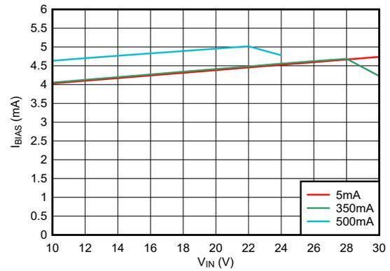
**Figure 5-4. Bias Current vs Input Voltage at  $T_J = 25^\circ\text{C}$  (New Chip)**
