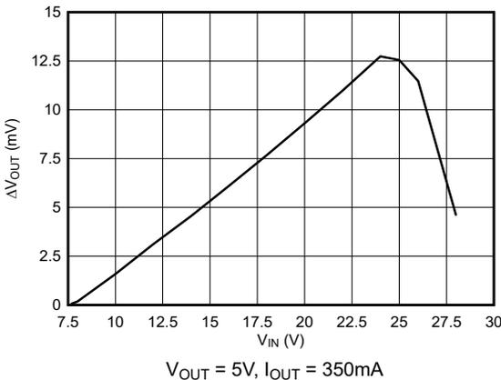
**Figure 5-3. Line Regulation at  $T_J = 25^\circ\text{C}$  (New Chip)**
