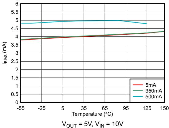
**Figure 5-5. Bias Current vs Temperature (New Chip)**
