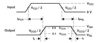
Figure 6-5. Propagation Delay Times
