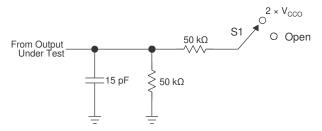
Figure 6-3. Load Circuit for Enable-Time and Disable-Time Measurement
