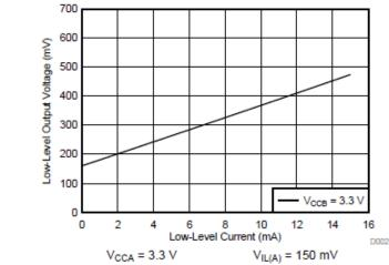
Figure 5-3. Low-Level Output Voltage  $(V_{OL(Bx)})$  vs Low-Level Current  $(I_{OL(Bx)})$
