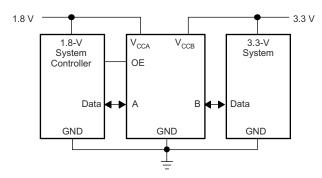
Figure 8-1. Typical Application Schematic
