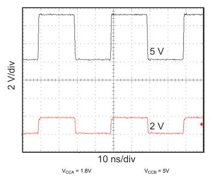
Figure 8-2. Level-Translation of a 2.5MHz Signal
