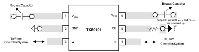
Figure 8-3. Typical Layout of TXS0101
