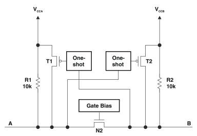
Figure 7-1. Architecture of a TXS01xx Cell
