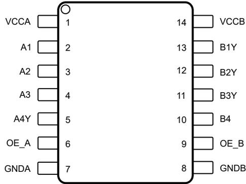
**Figure 4-3. TXG1041-Q1 DYY 14-Pin SOT Top View**
