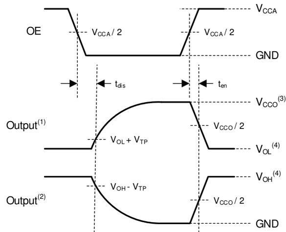
1. Output waveform on the condition that input is driven to a valid Logic Low.
