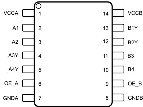
Figure 4-4. TXG1042-Q1 DYY 14-Pin SOT Top View
