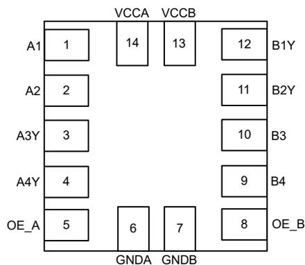
Figure 4-2. TXG1042-Q1 RUC Package 14-Pin X2QFN Top View
