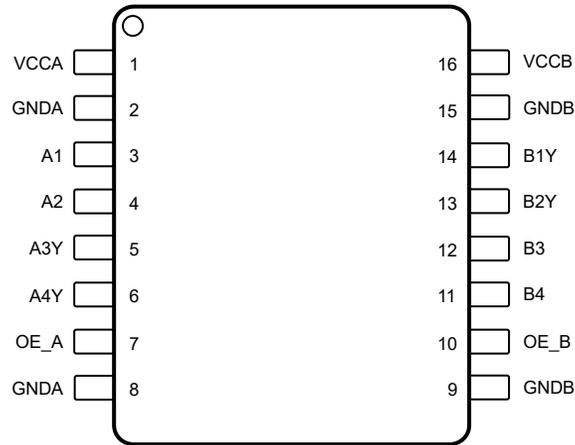
Figure 4-6. TXG1042-Q1 DBQ 16-Pin QSOP Top View
