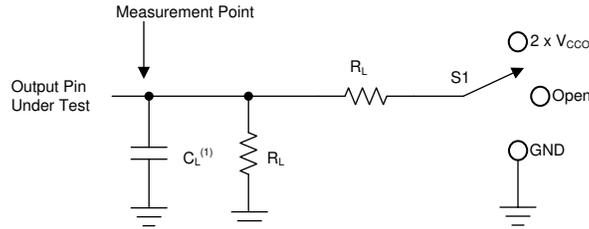
A.  $C_L$  includes probe and jig capacitance.
