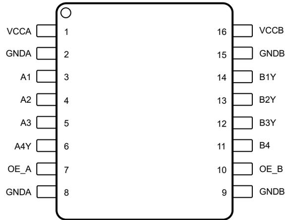
**Figure 4-5. TXG1041-Q1 DBQ 16-Pin QSOP Top View**
