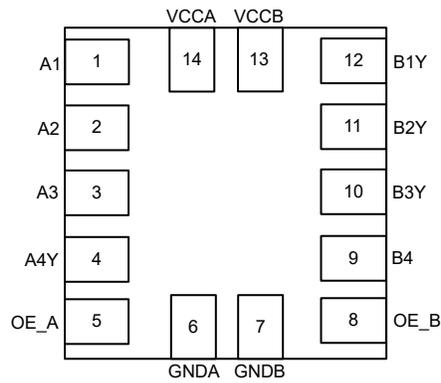
**Figure 4-1. TXG1041-Q1 RUC Package 14-Pin X2QFN Top View**
