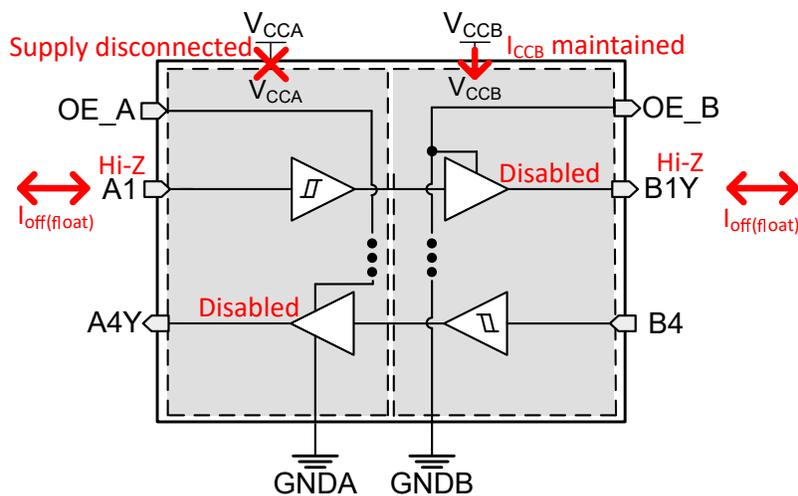
Figure 7-3. V<sub>CC</sub> Disconnect Feature
