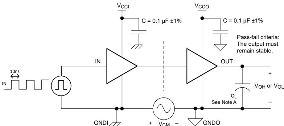
1.  $C_L = 15\text{pF}$  and includes instrumentation and fixture capacitance within  $\pm 20\%$ .
