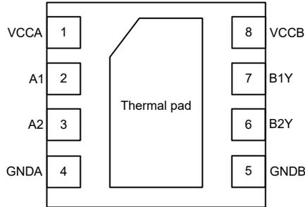
**Figure 4-2. TXGx020DSG Package 8-Pin WSON Top View**
