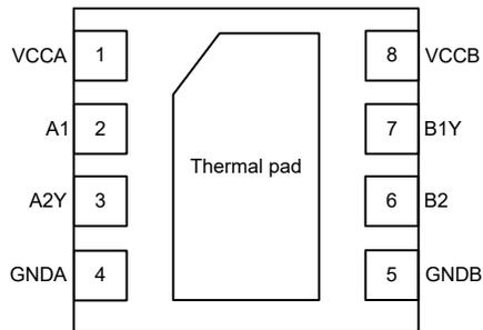
**Figure 4-1. TXGx021DSG Package 8-Pin WSON Top View**
