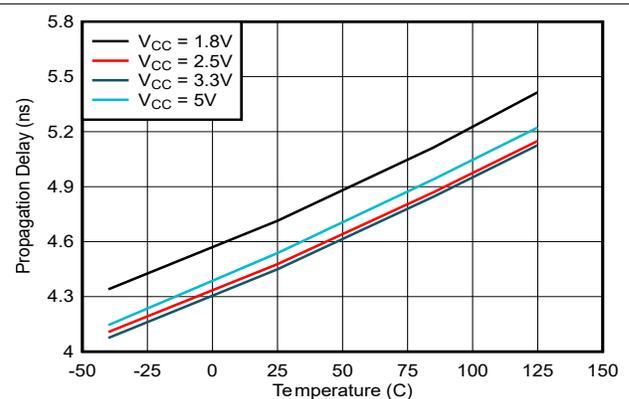
**Figure 6-6. Propagation Delay,  $T_{PLH}$ , vs Temperature**
