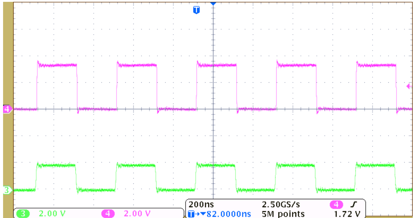
Figure 8-2. Example of Level Translation of a 2.5MHz 1.8V Signal (Green) to a 3.3V Signal (Pink)
