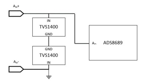
Figure 10. TVS1400 Application Schematic
