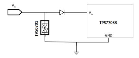
Figure 7. TVS0701 Application Schematic
