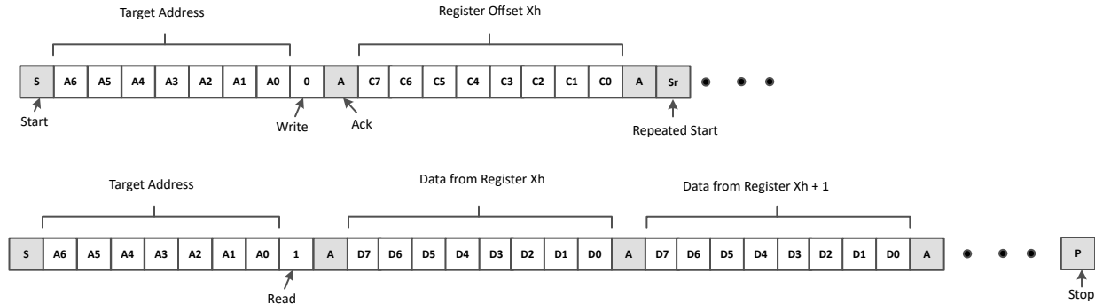
Figure 7-4. I 2 C Read with Repeated Start
