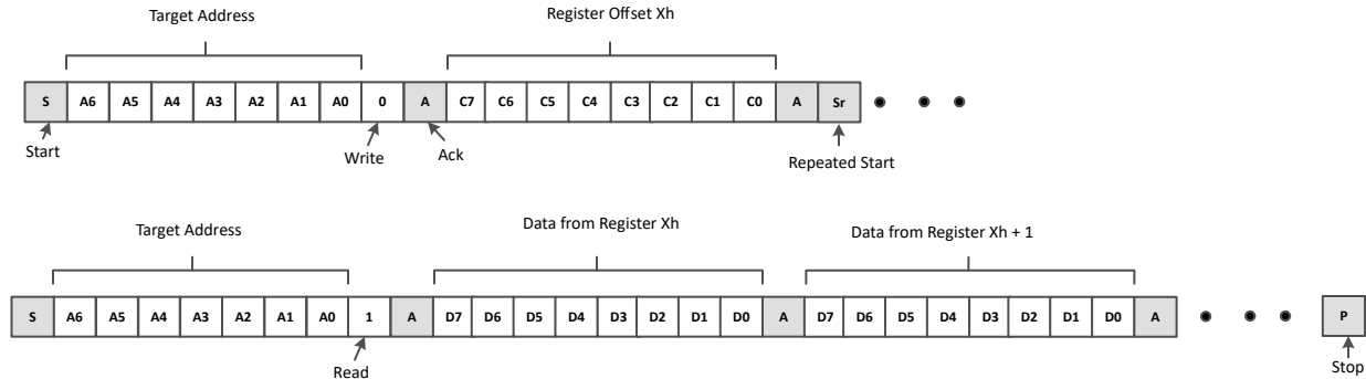
Figure 7-4. I 2 C Read with Repeated Start
