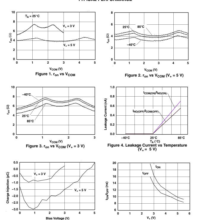
Figure 5. Charge-Injection (Q<sub>C</sub>) vs V<sub>COM</sub>
