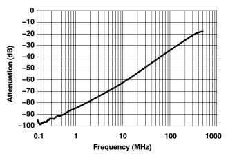
Figure 10. OFF Isolation vs Frequency
