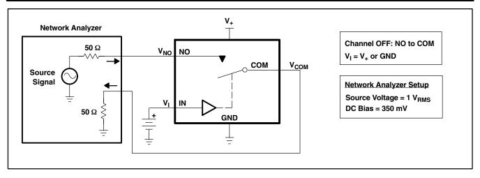
Figure 19. OFF Isolation (O<sub>ISO</sub>)
