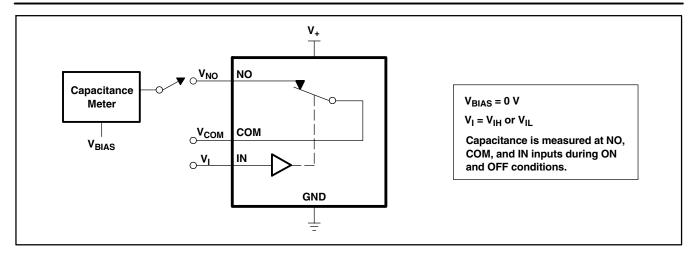
Figure 16. Capacitance (C<sub>I</sub>,  $C_{COM(OFF)}$ ,  $C_{COM(ON)}$ ,  $C_{NO(OFF)}$ ,  $C_{NO(ON)}$ )
