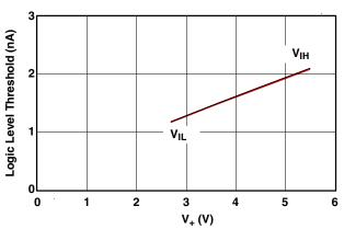
Figure 8. Logic-Level Threshold vs V<sub>+</sub>
