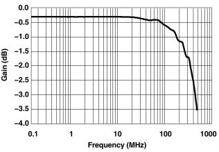
Figure 9. Bandwidth (Gain vs Frequency)  $(V_+ = 5 \text{ V})$
