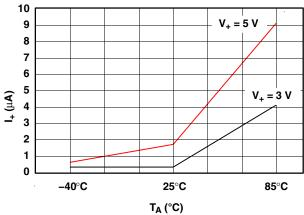
Figure 11. Power-Supply Current vs Temperature
