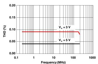
Figure 12. Total Harmonic Distortion vs Frequency
