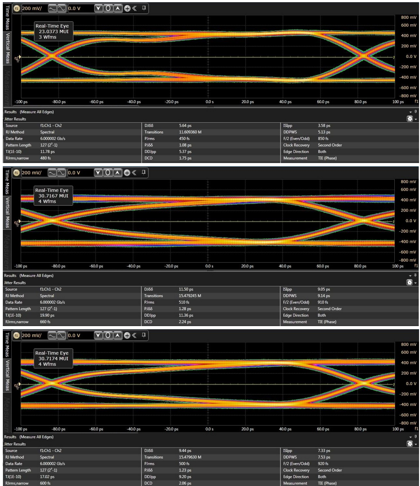
Figure 6-6. Typical eye diagrams at 6.0 Gbps. Top: baseline calibration setup. Middle: through TS3DV642-Q1 Port A. Bottom: through TS3DV642-Q1 Port B.
