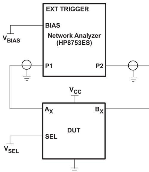
Figure 10. Test Circuit for Frequency Response (BW)
