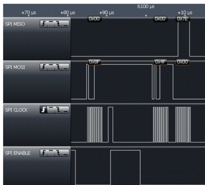
Figure 6-25. Reset FIFO and Read RSSI
