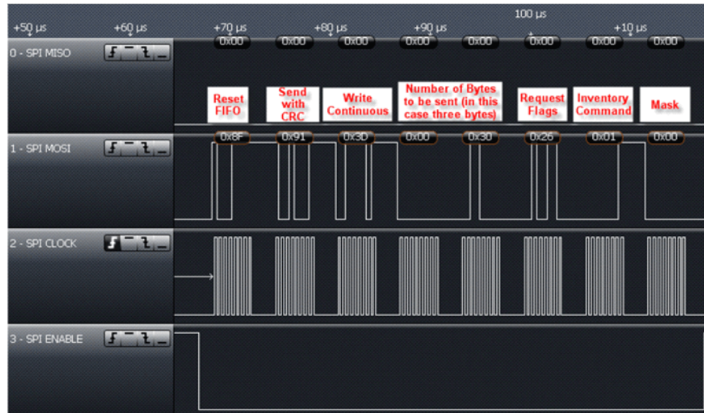
Figure 6-20. Inventory Command Sent From MCU to TRF7962A
