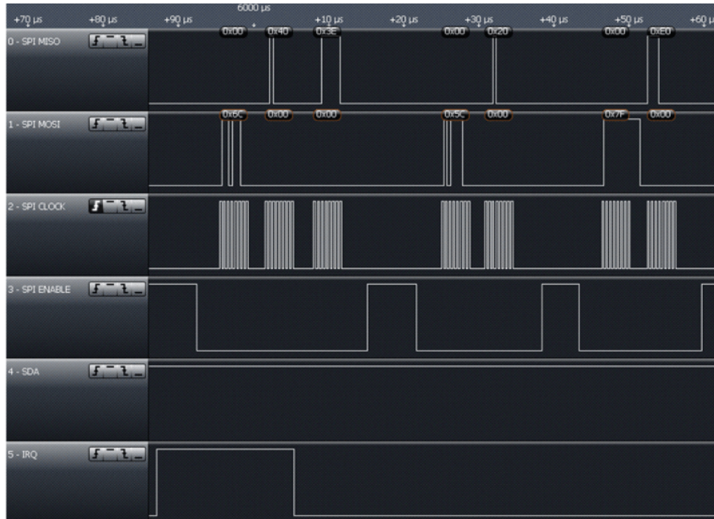
Figure 6-24. IRQ With One Byte in FIFO
