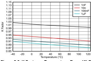
Figure 5-2. K Factor vs Temperature,  $R_{ext} = 10k\Omega$
