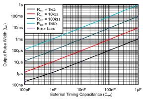
Figure 5-18. Typical output pulse width versus timing capacitance value with error bar overlay
