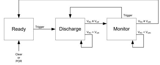
Figure 7-2. State Machine Diagram
