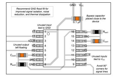
Figure 8-6. Layout Example for TPUL2G123 in the PW (TSSOP) package
