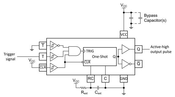
Figure 8-1. Pulse generator schematic using the TPUL2G123
