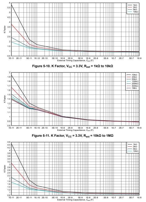
Figure 5-12. K Factor,  $V_{CC}$  = 5V,  $R_{ext}$  = 1k $\Omega$  to 10k $\Omega$
