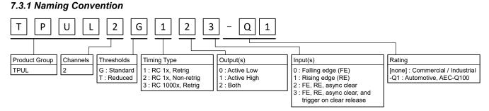
Figure 7-3. Device name meaning
