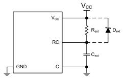
Figure 8-2. External protection diode connection
