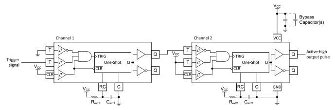
Figure 8-4. Delayed pulse generation schematic using the TPUL2G123
