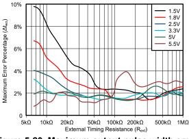
Figure 5-20. Maximum output pulse width error (absolute value) versus timing resistor values with (absolute value) versus timing resistor values with C<sub>ext</sub> = 100pF
