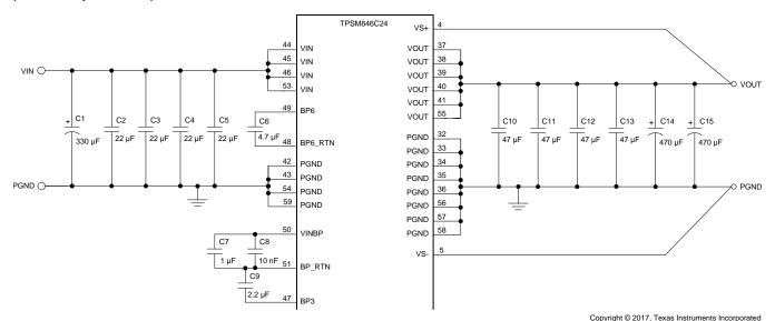
Figure 13. Required Capacitor Schematic
