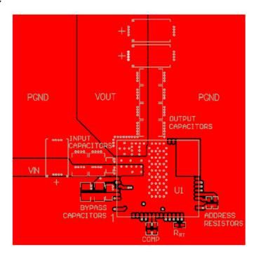
Figure 20. PCB Top-side Layout Recommendation
