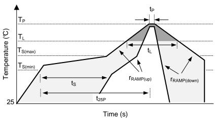
Figure 26. Recommended Reflow-Oven Thermal Profile
