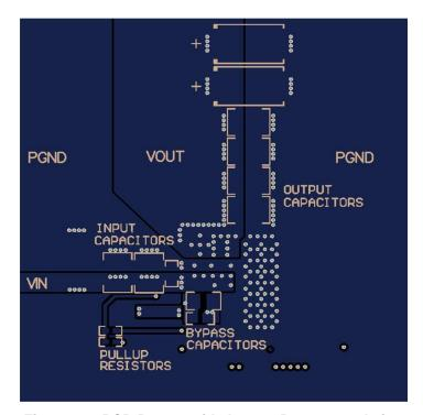
Figure 21. PCB Bottom-side Layout Recommendation
