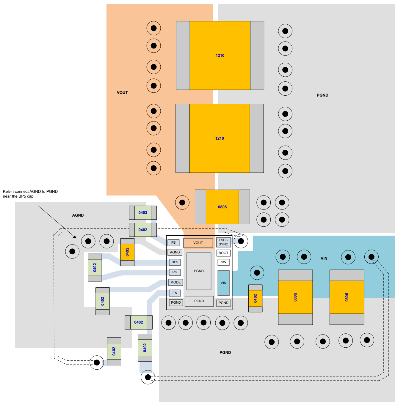
Figure 7-19. Example PCB Layout
