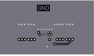
Figure 35. Typical GND Layer
