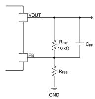
Figure 19. Feed-Forward Capacitor
