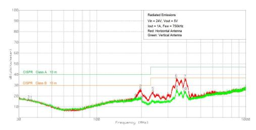
Figure 37. Radiated Emissions 24-V Input, 5-V Output, 1-A Load (EN55011 Class B)
