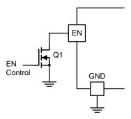
Figure 23. Typical Enable Control
