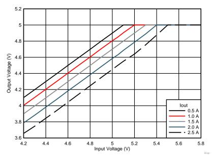
Figure 27. Voltage Dropout
