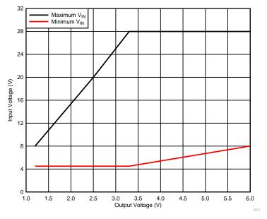
Figure 20. Input Voltage vs Output Voltage
