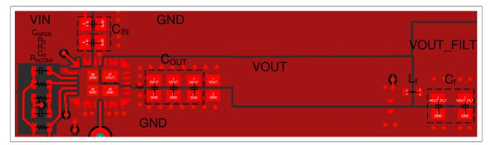
Figure 8-16. Recommended Layout for Design with Second L-C Filter
