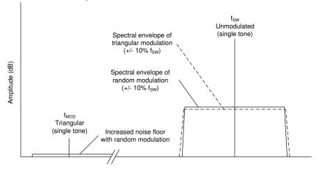
Figure 7-2. Spread Spectrum Modulation
