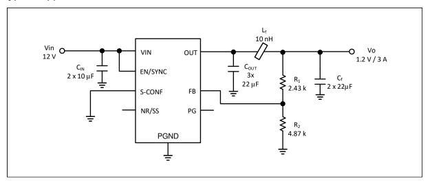
Figure 8-1. Typical Schematic
