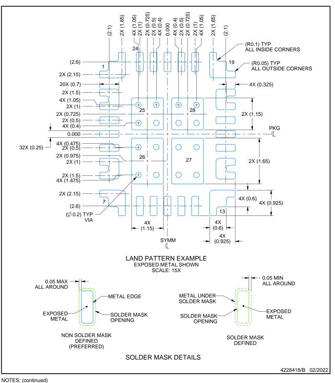
This package is designed to be soldered to a thermal pad on the board. For more information, see Texas Instruments literature number SLUA271 (www.ti.com/lit/slua271).
