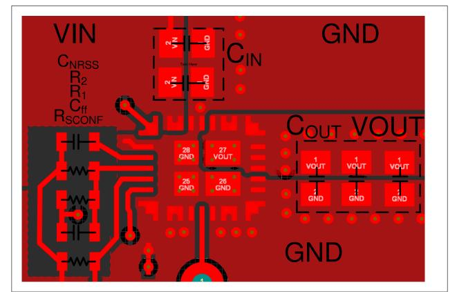
Figure 8-15. Recommended Layout for Single L-C Filter
