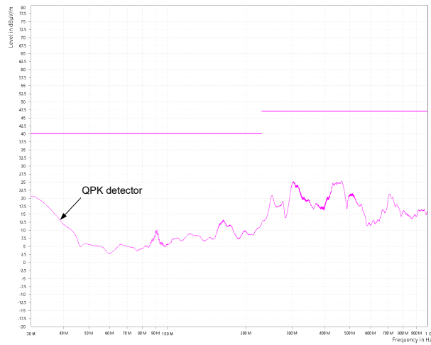
Figure 9-8. CISPR 32 Class B Radiated Emissions: Horizontal Polarization
