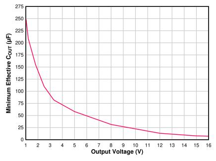
Figure 8-2. Minimum Required Output Capacitance
