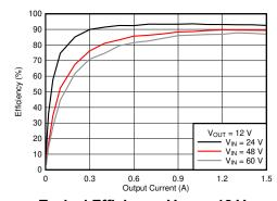
Typical Efficiency, V<sub>OUT</sub> = 12 V
