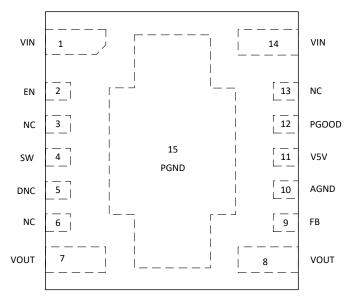
Figure 6-1. 15-Pin QFN RDA Package (Top View)
