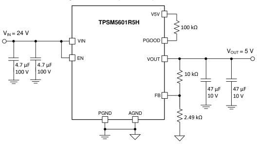
Figure 9-1. TPSM5601R5Hx Typical Schematic
