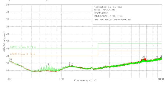
Figure 11-6. Radiated Emissions 24-V Input, 5-V Output, 1.5-A Load
