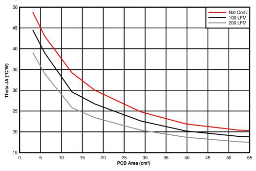
Figure 11-5.  $\theta_{JA}$  vs PCB Area
