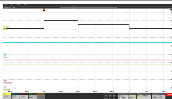
Figure 6-26. Slow Decrease and Slow Increase of Supply Voltage
