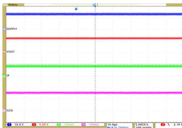
Figure 17. Constant Output Current With Heat Sharing Resistor
