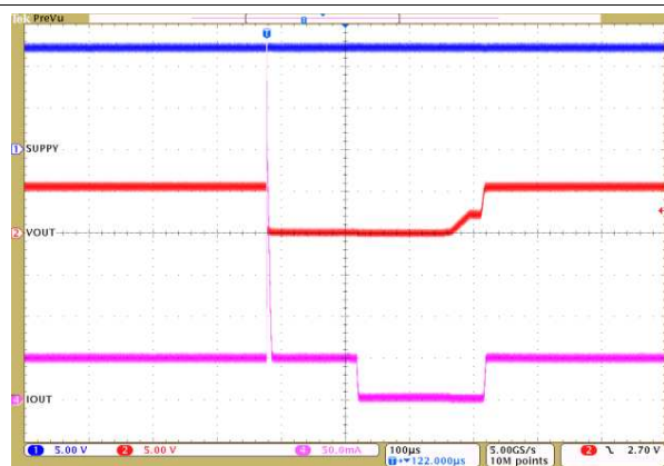
Figure 11. LED Short-Circuit Protection and Recovery
