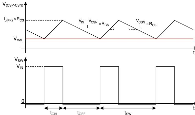
**Figure 7-1. Adaptive On Time Control Buck Converter Waveforms**
