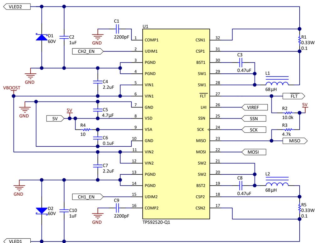
Figure 8-3. Application Schematic
