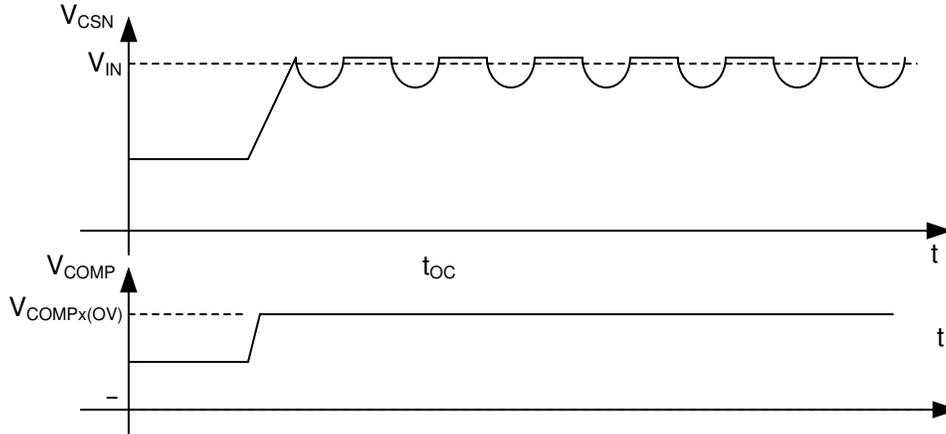
**Figure 7-10. Open Circuit Condition with Output Voltage Oscillation**
