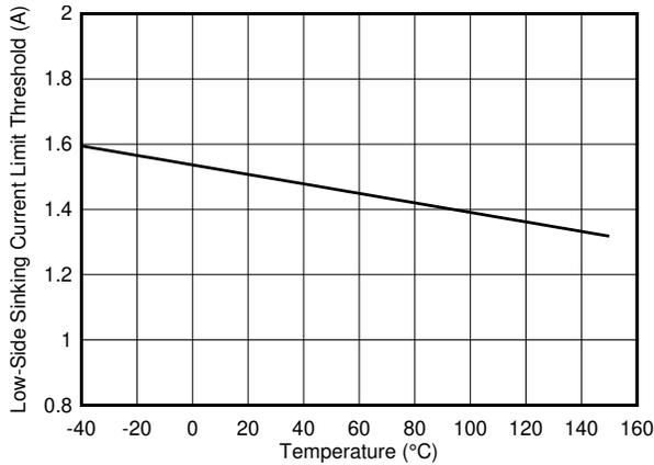
**Figure 6-13. Low-Side Sinking Current Limit Threshold vs Temperature**
