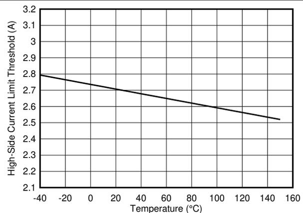
Figure 6-11. High-Side Current Limit Threshold vs Temperature
