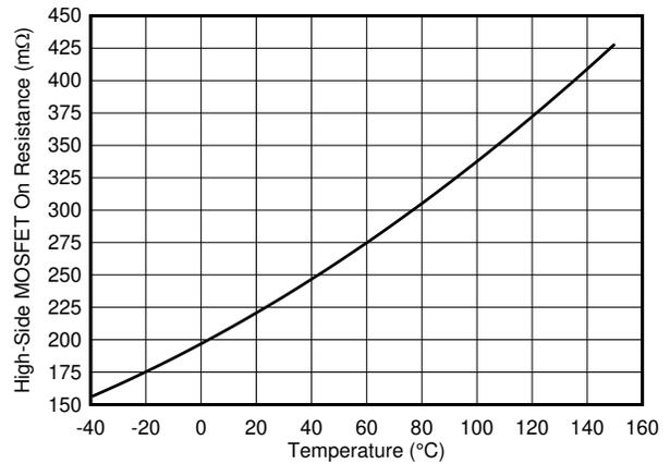
Figure 6-8. High Side MOSFET On Resistance vs Temperature
