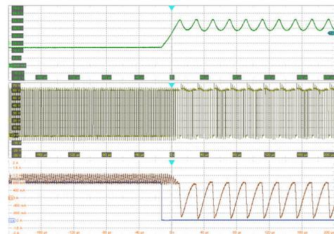
Ch1: SW voltage (10V/div); Ch2: Output voltage (4 V/div); Ch3: Inductor current
