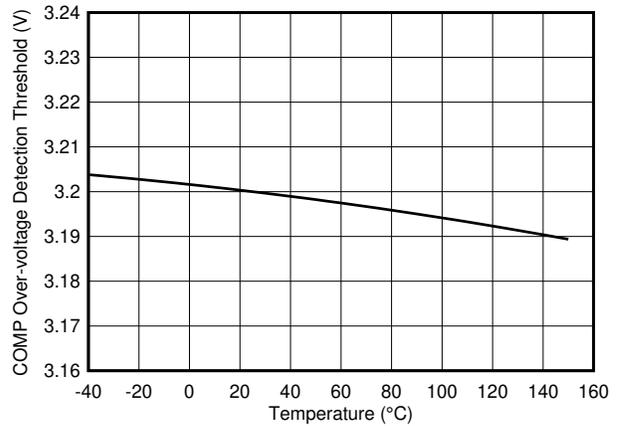
Figure 6-20. COMP Over-voltage Detection Threshold vs Temperature
