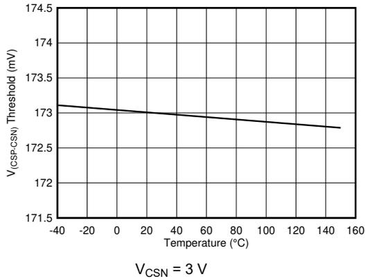
Figure 6-1.  $V_{(CSP-CSN)}$  Current Sense Threshold vs Temperature
