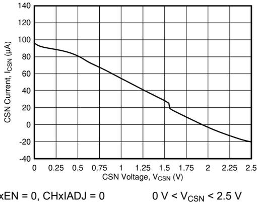
Figure 6-3. CSN Source Current vs CSN Voltage
