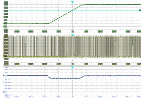
Ch1: SW voltage (10 V/div); Ch2: Output voltage (4 V/div);
