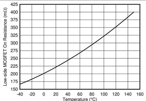
Figure 6-12. Low-Side MOSFET On Resistance vs Temperature
