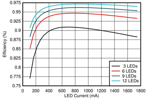
$V_{IN} = 60\text{ V}$   $f_{SW} = 437\text{ kHz}$
