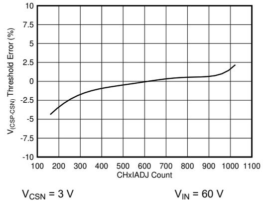
Figure 6-2.  $V_{(CSP-CSN)}$  Current Sense Error vs IADJ Count
