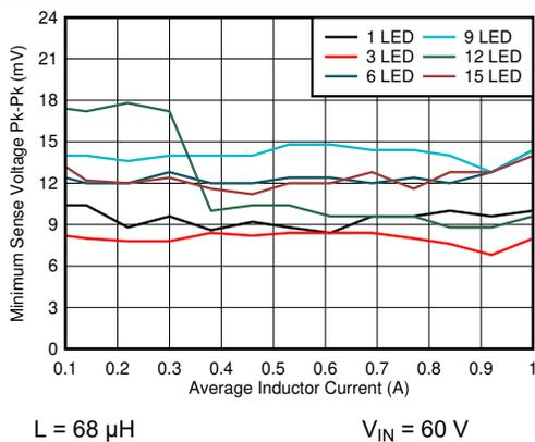
Figure 6-5. Minimum Ripple Voltage vs Average Inductor Current
