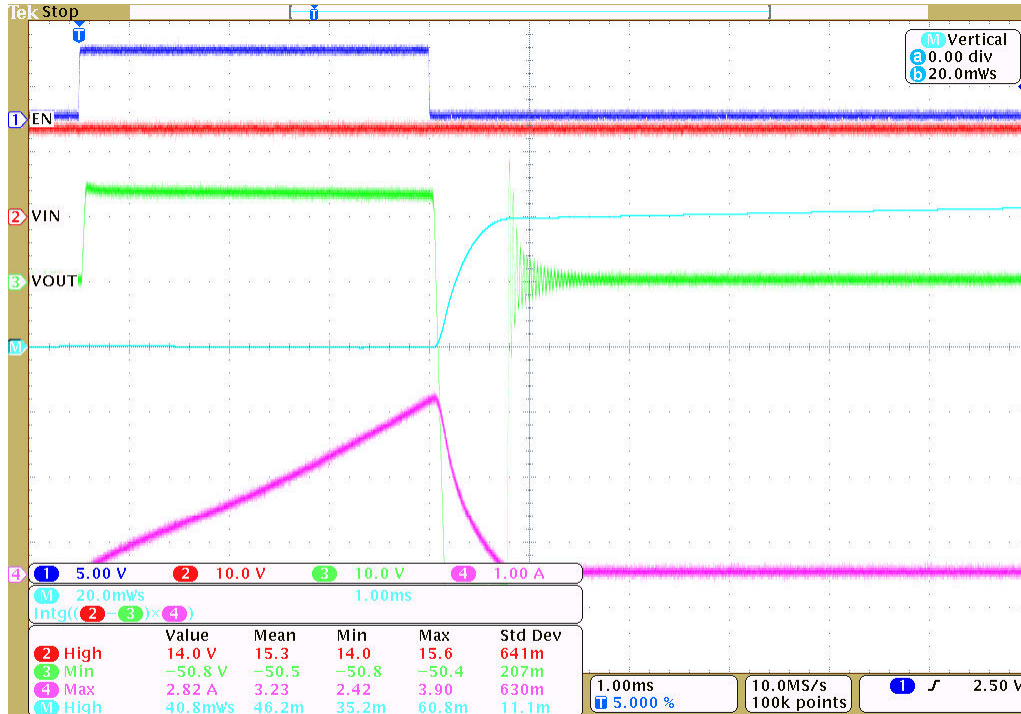
Figure 8-7. Inductive Load Switching-Off Waveform of 40mJ
