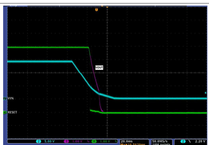
Figure 24. TPS7B6750-Q1 Power-Down Waveform
