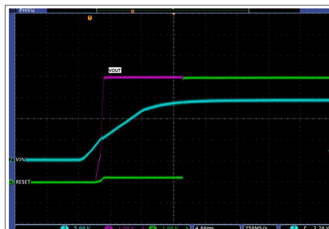
Figure 23. TPS7B6750-Q1 Power-Up Waveform
