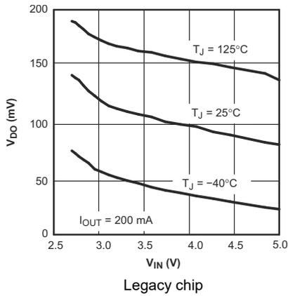
**Figure 5-31. TPS793 Dropout Voltage vs Input Voltage**
