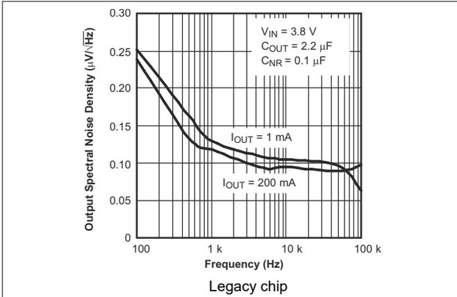
Figure 5-7. TPS793 Output Spectral Noise Density vs Frequency
