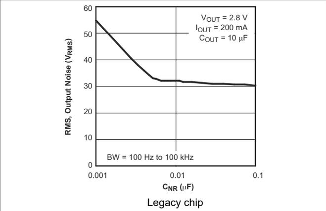
Figure 5-10. Root Mean Square Output Noise vs  $C_{NR}$
