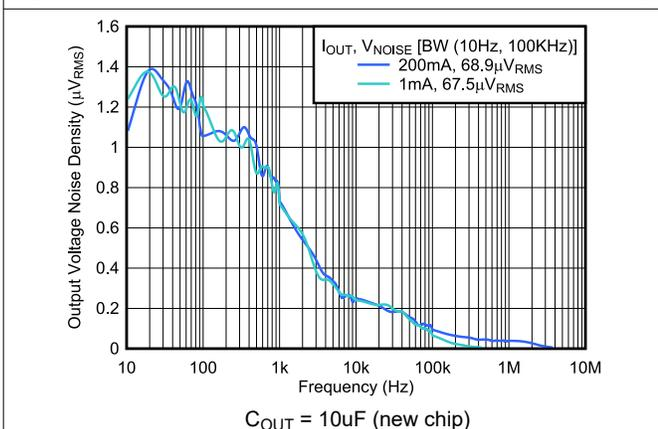
Figure 5-11. TPS793 Output Spectral Noise Density vs Frequency
