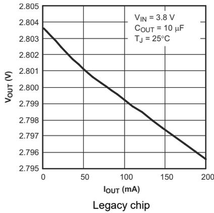
Figure 5-1. TPS793 Output Voltage vs Output Current
