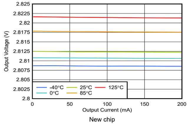
Figure 5-2. TPS793 Output Voltage vs Output Current
