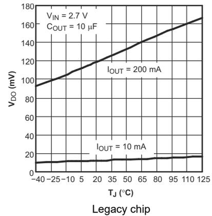
Figure 5-14. TPS793 Dropout Voltage vs Junction Temperature
