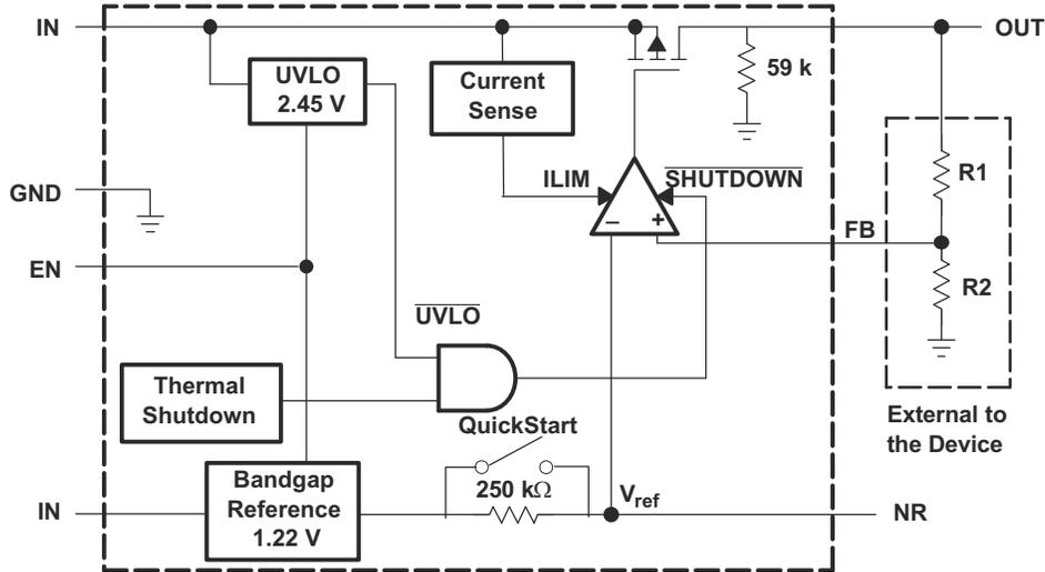
Figure 6-1. TPS79301 Block Diagram (Adjustable Version, Legacy Chip)
