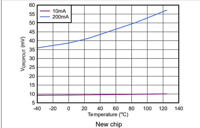
Figure 5-15. TPS793 Dropout Voltage vs Junction Temperature
