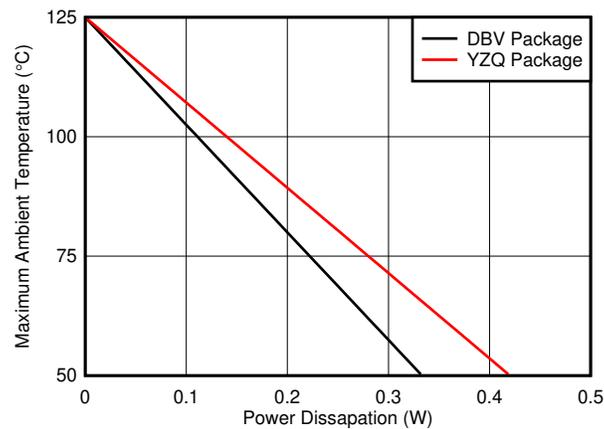
**Figure 7-8. Maximum Ambient Temperature vs Power Dissipation**
