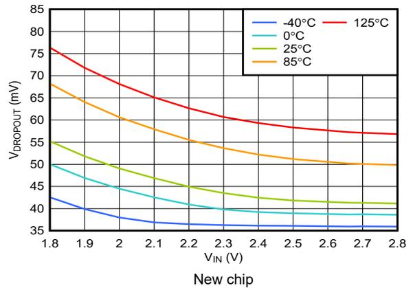
**Figure 5-32. TPS793 Dropout Voltage vs Input Voltage**
