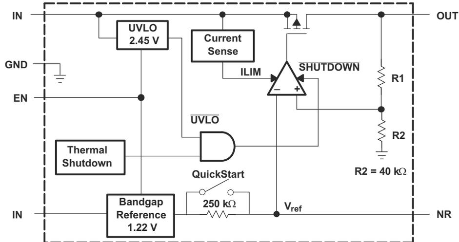
Figure 6-2. TPS793 Block Diagram (Fixed Version, Legacy Chip)
