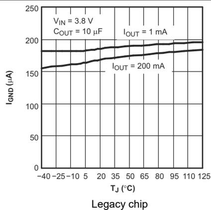
Figure 5-5. TPS793 Ground Current vs Junction Temperature
