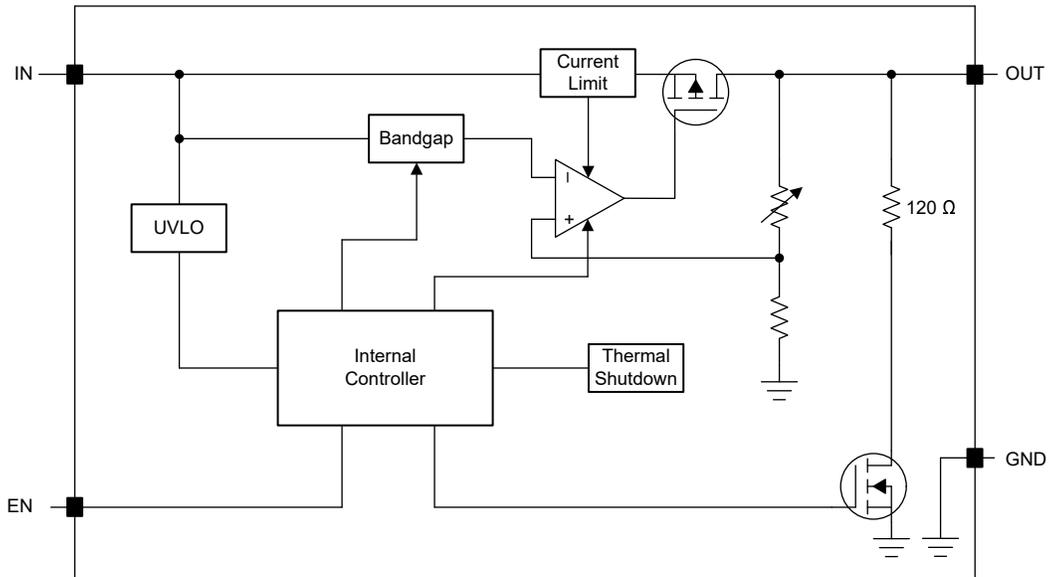
**Figure 6-4. TPS793 Block Diagram (Fixed Version, New Chip)**
