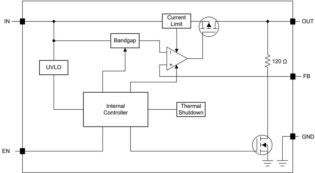
**Figure 6-3. TPS79301 Block Diagram (Adjustable Version, Legacy Chip)**
