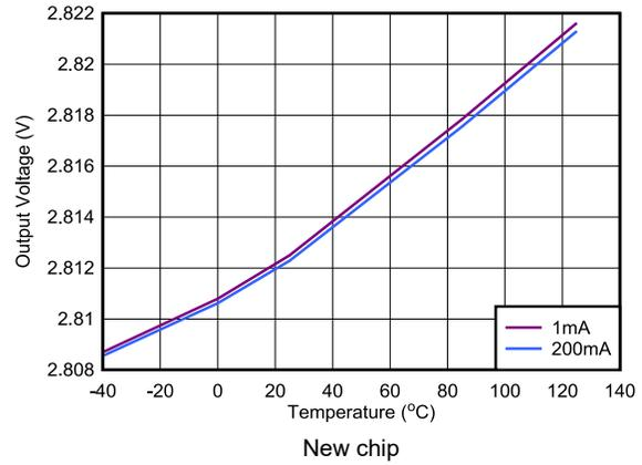
Figure 5-4. TPS793 Output Voltage vs Junction Temperature
