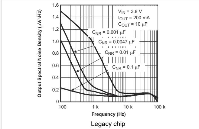
Figure 5-9. TPS793 Output Spectral Noise Density vs Frequency
