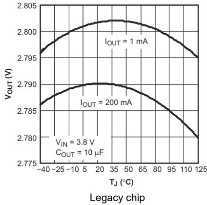
Figure 5-3. TPS793 Output Voltage vs Junction Temperature
