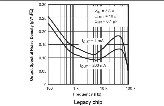
Figure 5-8. TPS793 Output Spectral Noise Density vs Frequency
