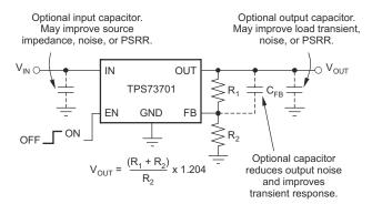
Figure 7-2. Typical Application Circuit For Adjustable-Voltage Version
