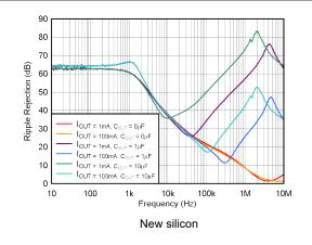
Figure 5-24. PSRR (Ripple Rejection) vs Frequency
