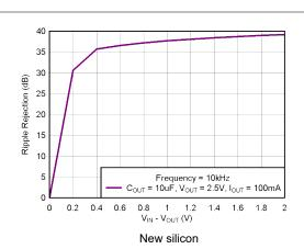
Figure 5-26. PSRR (Ripple Rejection) vs (V<sub>IN</sub> - V<sub>OUT</sub>)
