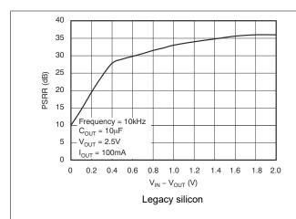
Figure 5-25. PSRR (Ripple Rejection) vs  $V_{IN}$  –  $V_{OUT}$
