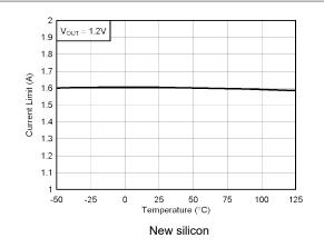
Figure 5-21. Current Limit vs Temperature
