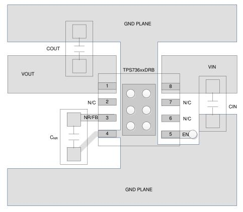
Figure 7-8. Fixed Output Voltage Option Layout (DRB Package)
