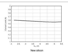
Figure 5-20. Current Limit vs VIN
