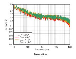
Figure 5-28. Noise Spectral Density
