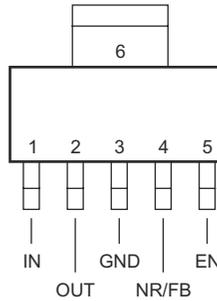
Figure 4-3. DCQ Package, 6-Pin SOT-223 (Top View)
