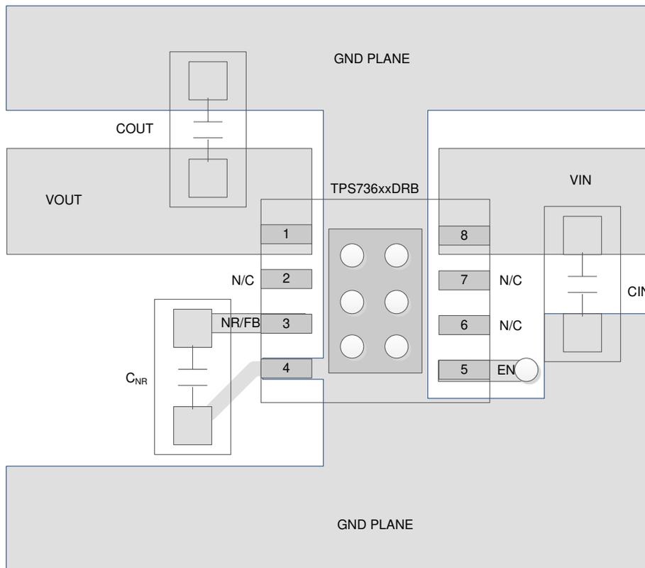
**Figure 7-11. Fixed Output Voltage Option Layout (DRB Package)**
