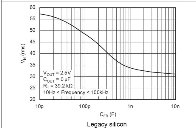
Figure 7-7. TPS73601 RMS Noise Voltage vs  $C_{FB}$
