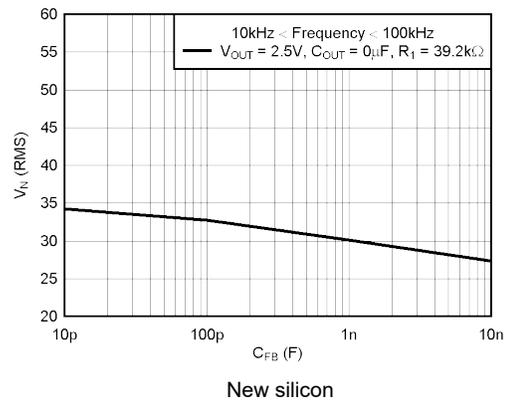
Figure 5-48. TPS73601 RMS Noise Voltage vs  $C_{FB}$
