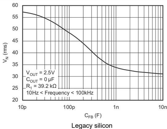
Figure 5-47. TPS73601 RMS Noise Voltage vs  $C_{FB}$
