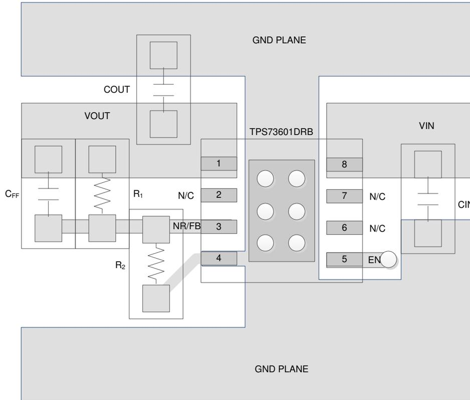
**Figure 7-12. Adjustable Output Voltage Option Layout (DRB Package)**
