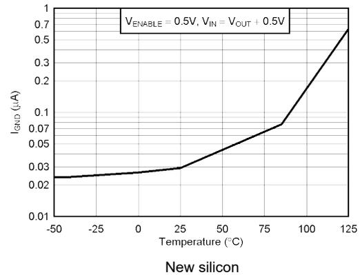
**Figure 5-16. Ground Pin Current in Shutdown vs Temperature**
