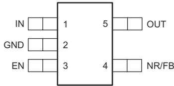
Figure 4-1. DBV Package, 5-Pin SOT-23 (Top View)
