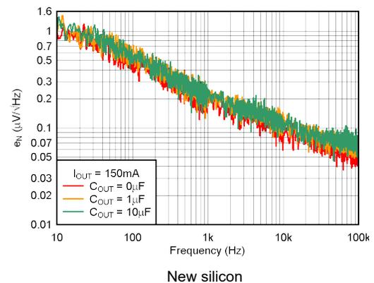
**Figure 5-30. Noise Spectral Density  $C_{NR} = 0.01\mu\text{F}$**
