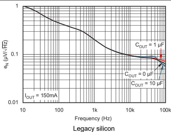
**Figure 5-29. Noise Spectral Density  $C_{NR} = 0.01\mu\text{F}$**
