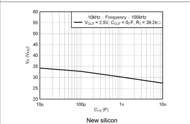
Figure 7-8. TPS73601 RMS Noise Voltage vs  $C_{FB}$
