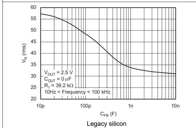
Figure 7-7. TPS73201 RMS Noise Voltage vs C<sub>FB</sub>
