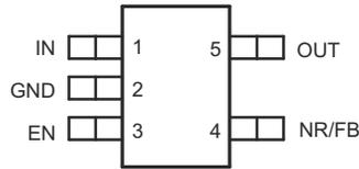
Figure 4-1. DBV Package, 5-Pin SOT-23 (Top View)
