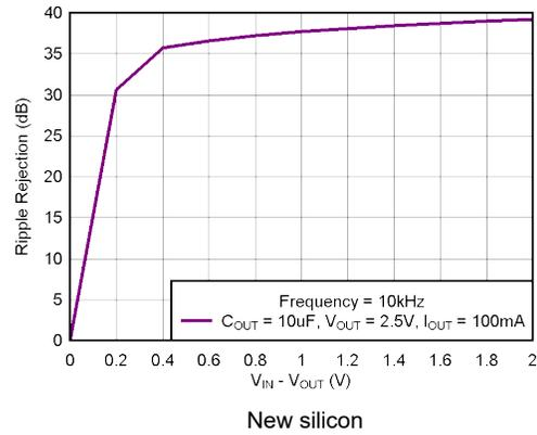
**Figure 5-26. PSRR (Ripple Rejection) vs ( $V_{IN} - V_{OUT}$ )**
