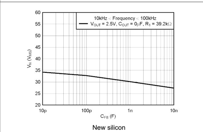
Figure 7-8. TPS73201 RMS Noise Voltage vs C<sub>FB</sub>
