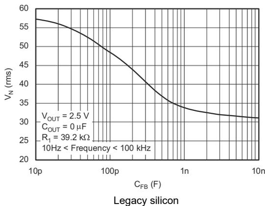
Figure 5-47. TPS73201 RMS Noise Voltage vs  $C_{FB}$
