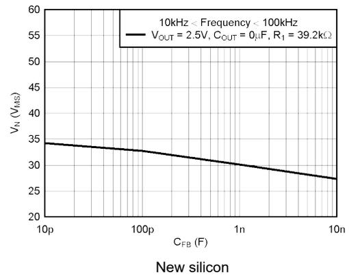
Figure 5-48. TPS73201 RMS Noise Voltage vs  $C_{FB}$
