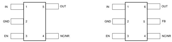
Figure 4-1. DBV Package, 5-Pin SOT-23 Fixed-Voltage Version (Top View)
