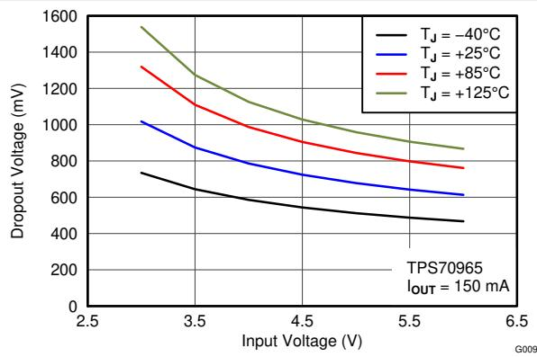
Figure 6-9. Dropout Voltage vs  $V_{\text{IN}}$  and Temperature
