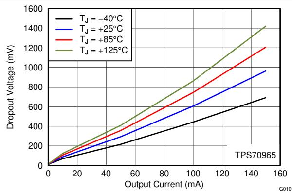
Figure 6-10. Dropout Voltage vs  $I_{\text{OUT}}$  and Temperature
