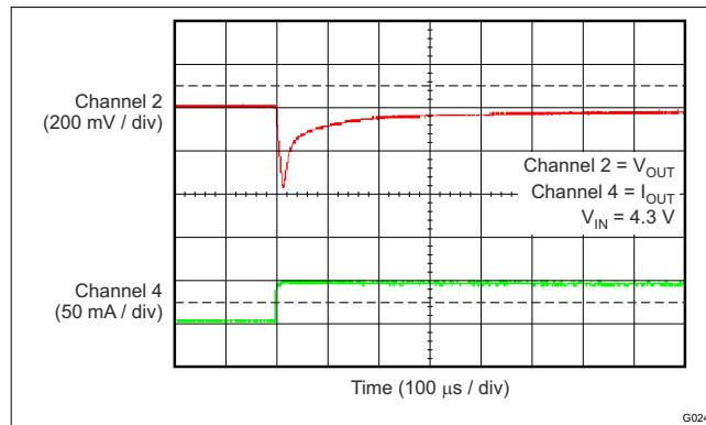
**Figure 6-25. TPS70933 Load Transient
