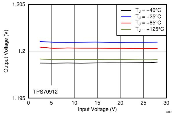
Figure 6-1. 1.2-V Line Regulation vs  $V_{\text{IN}}$  and Temperature
