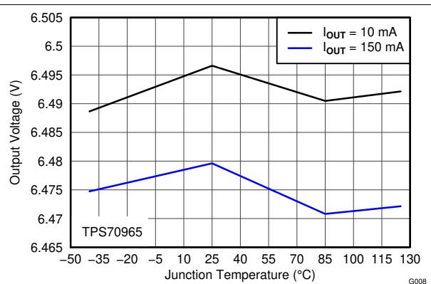
Figure 6-8.  $V_{\text{OUT}}$  vs Temperature
