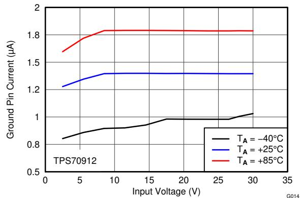
Figure 6-14. GND Current vs  $V_{\text{IN}}$  and Temperature
