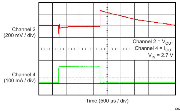
Figure 6-22. TPS70912 Load Transient
