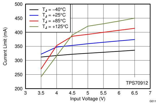
Figure 6-11. 1.2-V Current Limit vs  $V_{\text{IN}}$  and Temperature
