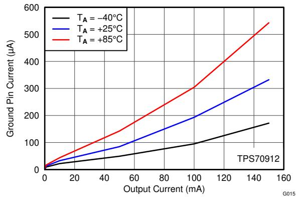
Figure 6-16. GND Current vs  $I_{\text{OUT}}$  and Temperature
