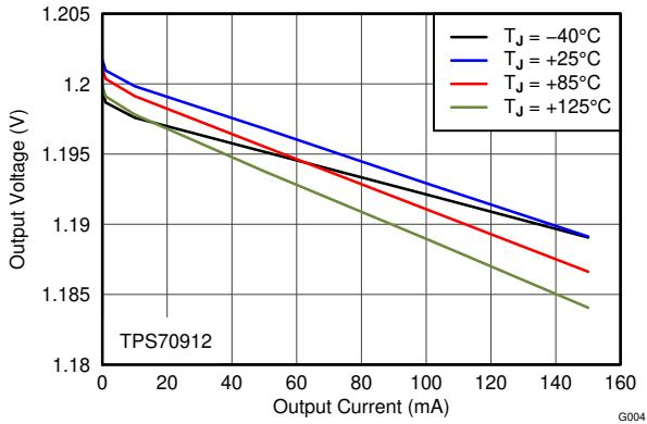
Figure 6-4. 1.2-V Load Regulation vs  $I_{\text{OUT}}$  and Temperature
