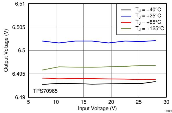
Figure 6-3. 6.5-V Line Regulation vs  $V_{\text{IN}}$  and Temperature
