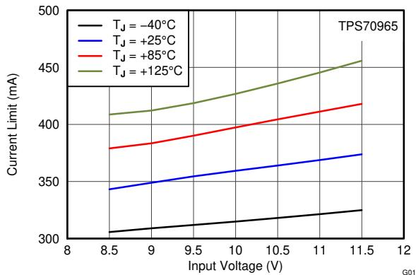
Figure 6-13. 6.5-V Current Limit vs  $V_{\text{IN}}$  and Temperature
