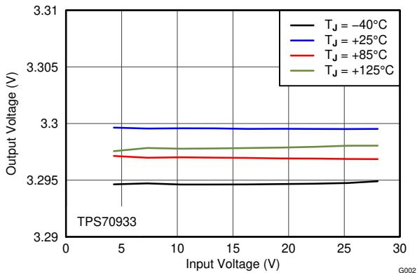
Figure 6-2. 3.3-V Line Regulation vs  $V_{\text{IN}}$  and Temperature
