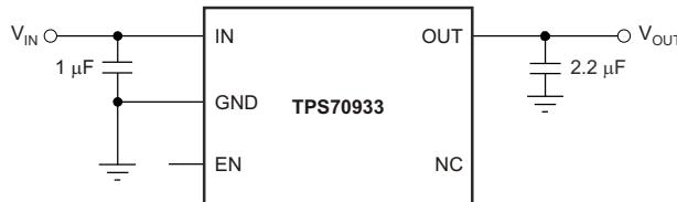
Figure 8-1. Wide Input, 3.3-V, Low- $I_Q$  Rail
