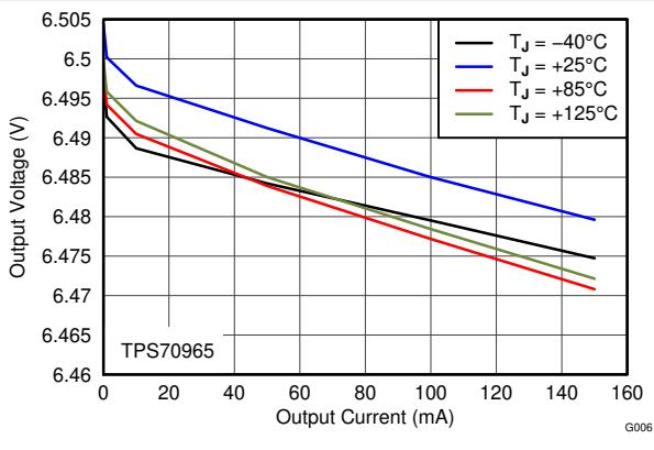
Figure 6-6. 6.5-V Load Regulation vs  $I_{\text{OUT}}$  and Temperature
