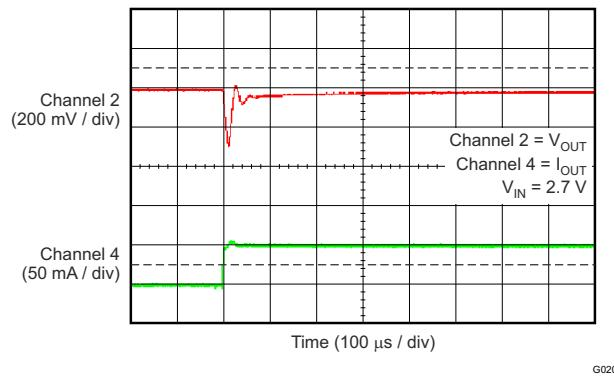
Figure 6-21. TPS70912 Load Transient
