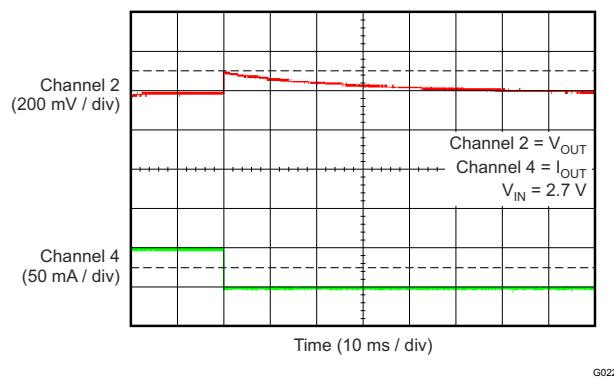
Figure 6-23. TPS70912 Load Transient
