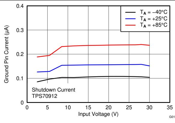
Figure 6-17. Shutdown Current vs  $V_{\text{IN}}$  and Temperature
