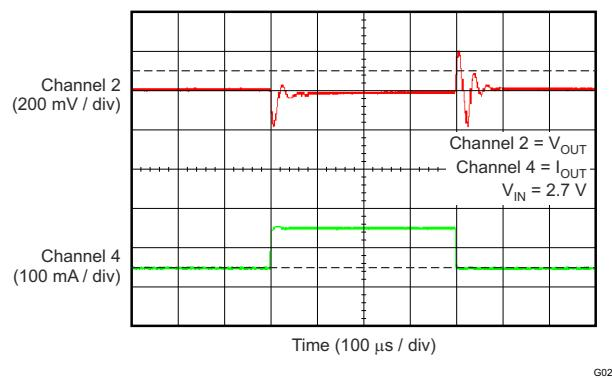
Figure 6-24. TPS70912 Load Transient
