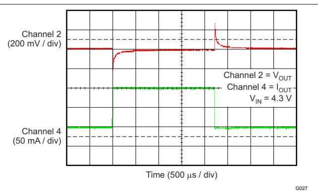
**Figure 6-28. TPS70933 Load Transient
