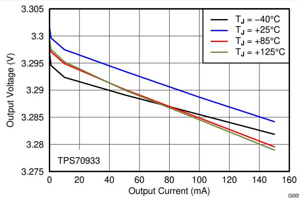
Figure 6-5. 3.3-V Load Regulation vs  $I_{\text{OUT}}$  and Temperature
