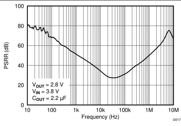
Figure 6-18. Power-Supply Rejection Ratio vs Frequency
