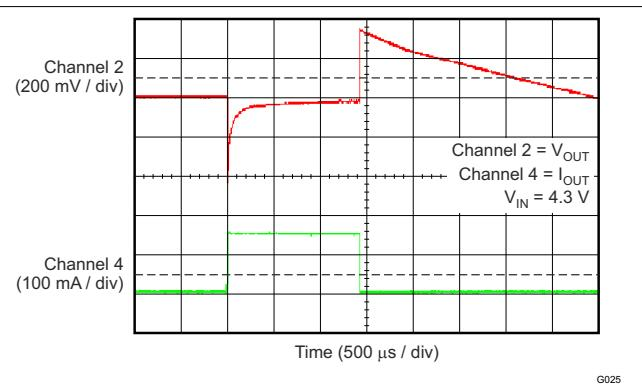
**Figure 6-26. TPS70933 Load Transient
