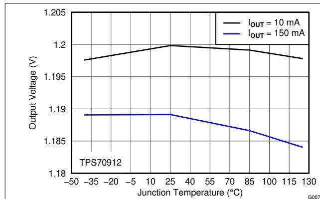
Figure 6-7.  $V_{\text{OUT}}$  vs Temperature
