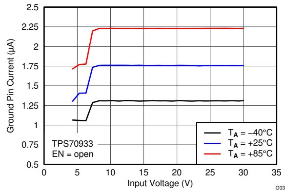
Figure 6-15. GND Current vs  $V_{\text{IN}}$  and Temperature
