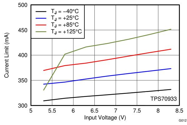
Figure 6-12. 3.3-V Current Limit vs  $V_{\text{IN}}$  and Temperature
