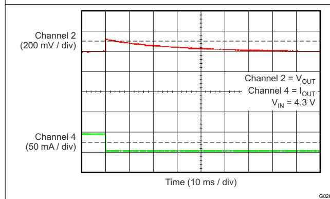
**Figure 6-27. TPS70933 Load Transient
