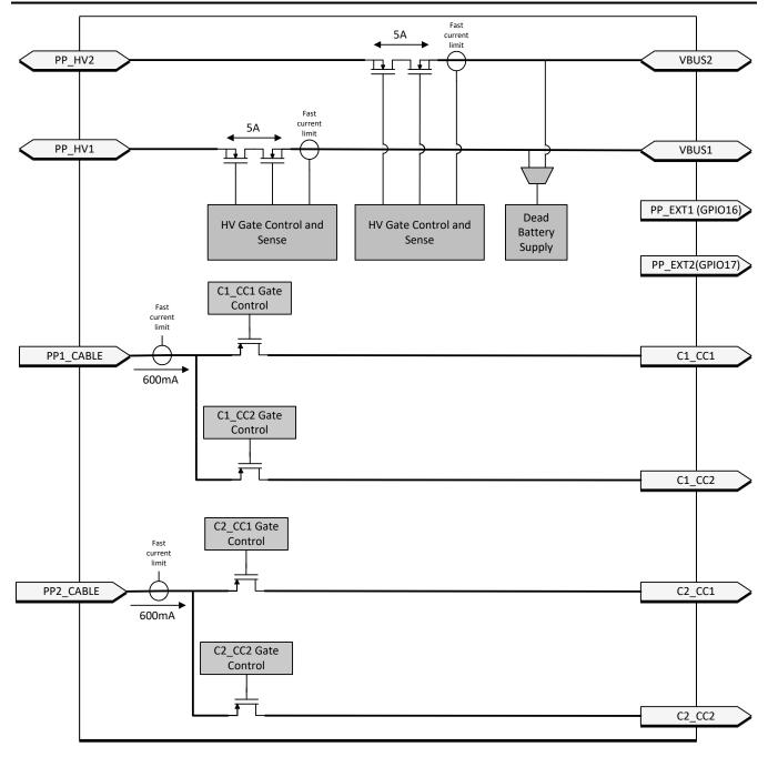
Figure 8-10. Port Power Switches
