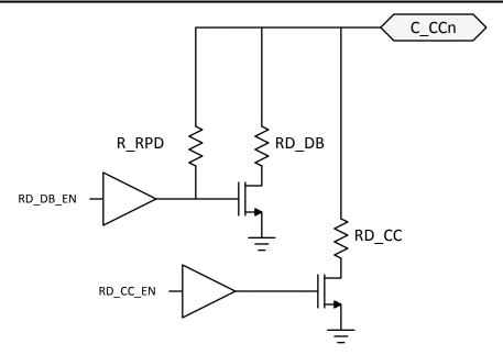
Figure 8-16. Dead Battery Pull-Down Resistor
