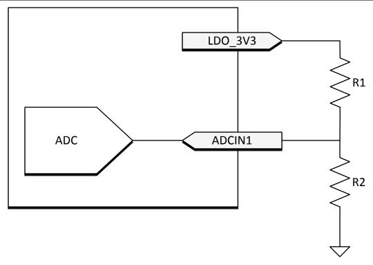
Figure 8-17. ADCIN1 Resistor Divider
