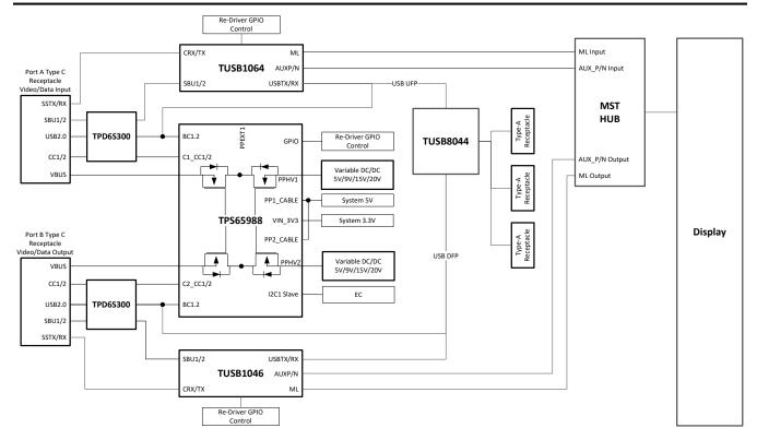
Figure 9-11. USB and DisplayPort Dock Block Diagram
