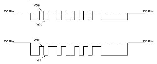
Figure 8-6. TX Driver Transmission with DC Bias
