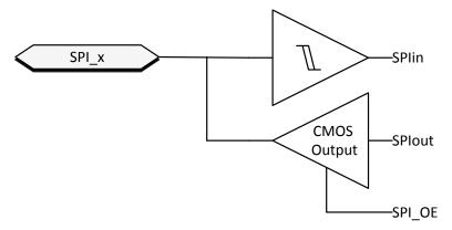
Figure 8-21. SPI buffer
