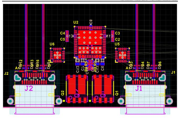
Figure 11-13. Protection Placement
