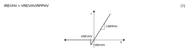
Figure 8-11. Comparator Mode (Source) Internal HV Switch I-V Curve
