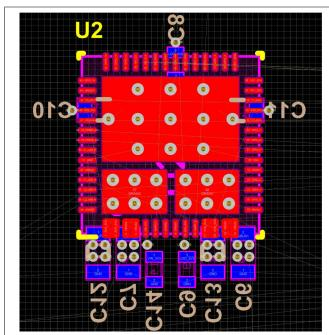
Figure 11-9. System Capacitors Placement Top/ Bottom Layer
