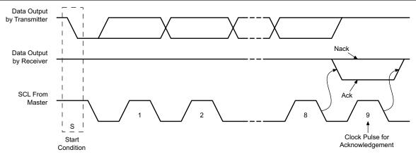
Figure 8-25. I<sup>2</sup>C Acknowledgment
