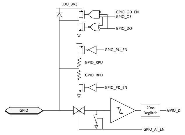
Figure 8-19. General GPIO Buffer
