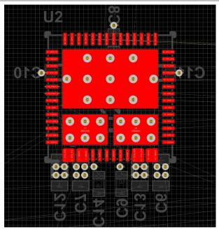
Figure 11-10. System Capacitors Placement Top Layer
