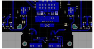
Figure 11-21. VBUS Routing Bottom Layer
