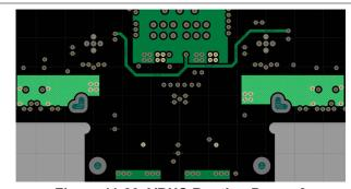
Figure 11-20. VBUS Routing Power 2
