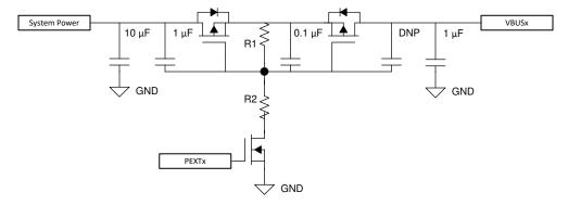
Figure 9-2. Simple Sink Power Path
