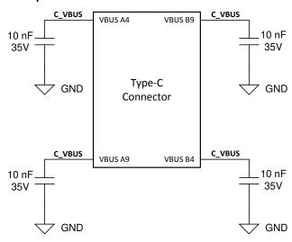
Figure 9-3. Type-C Connector VBUS Capacitors
