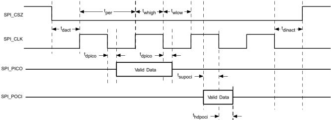
Figure 7-2. SPI Controller Timing
