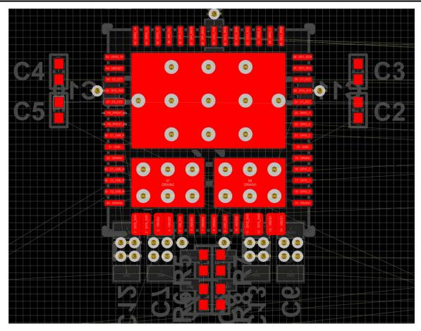
Figure 11-12. CC and ADCIN1/2 Component Placements
