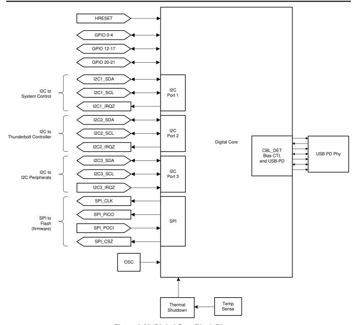
Figure 8-22. Digital Core Block Diagram
