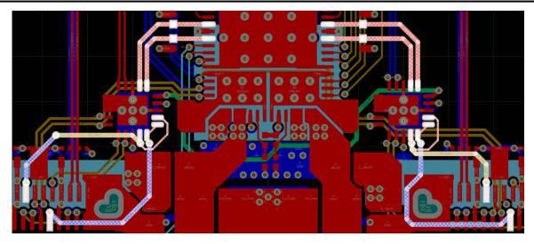
Figure 11-14. Complete CC Routing
