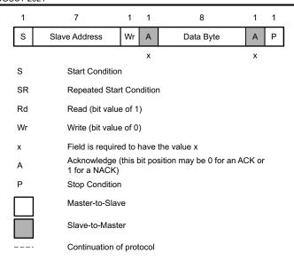
Figure 8-28. I<sup>2</sup>C Read/Write Protocol Key
