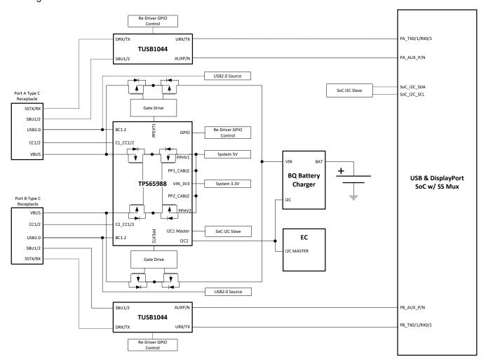
Figure 9-9. TPS65988 and SoC I2C with Re-Driver GPIO
