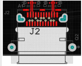
Figure 11-7. Type-C Connector SSTXRX Top Layer
