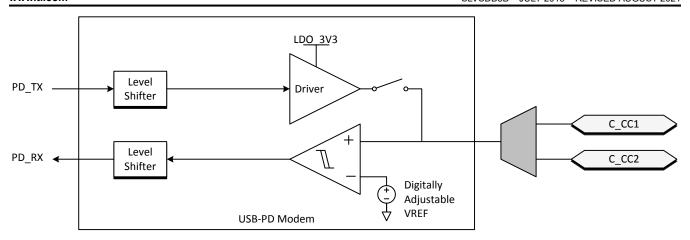
Figure 8-5. USB-PD BMC TX/Rx Block Diagram
