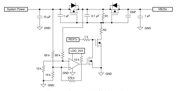
Figure 9-1. Recommended Sink Power Path
