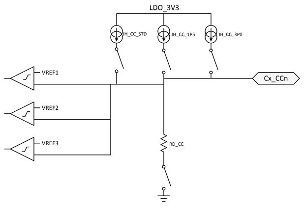
Figure 8-14. Plug and Orientation Detection Block
