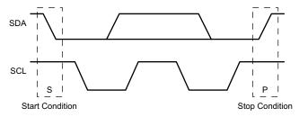
Figure 8-23. I<sup>2</sup>C Definition of Start and Stop Conditions
