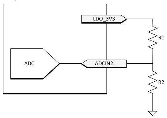
Figure 8-29. I<sup>2</sup>C Address Divider
