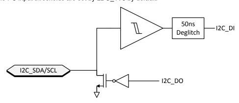
Figure 8-20. I<sup>2</sup>C Buffer
