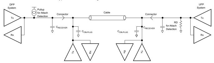
Figure 8-8. Example USB-PD Multi-Drop Configuration
