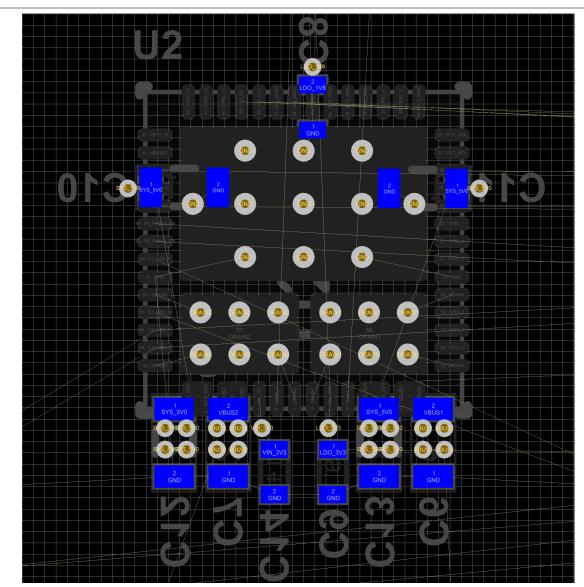
Figure 11-11. System Capacitors Placement Bottom Layer
