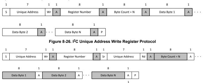
Figure 8-27. I<sup>2</sup>C Unique Address Read Register Protocol
