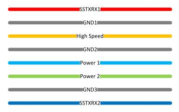
Figure 11-3. 8 Layer Board Stack Up
