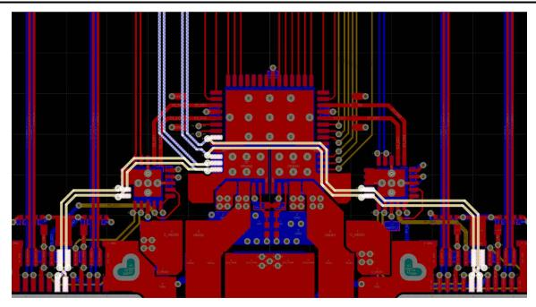
Figure 11-17. Complete USB2 Routing
