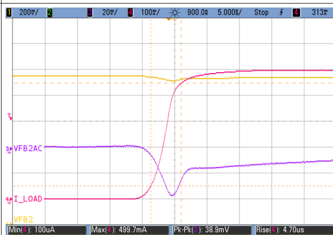
Figure 7-5. VDD2 Rising Load Transient Response
