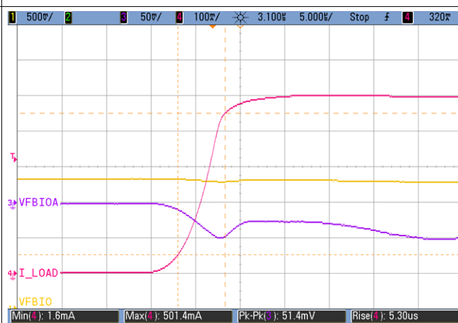
Figure 7-5. VDD2 Rising Load Transient Response
