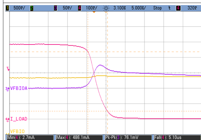
Figure 7-4. VDD2 Falling Load Transient Response
