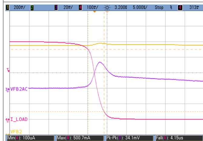
Figure 7-4. VDD2 Falling Load Transient Response
