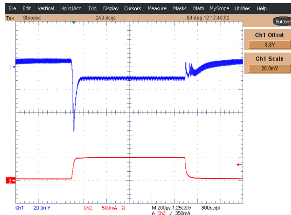
Figure 76. DCDCx Load Transient Response, 3.3 V OUT , 50-500-50 mA Load
