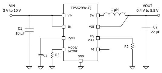
Figure 8-3. Selectable V<sub>O</sub> Operation Schematic
