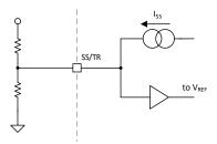
Figure 8-4. Tracking Operation Simplified Schematic
