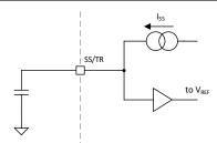
Figure 9-2. Soft-Start Operation Simplified Schematic
