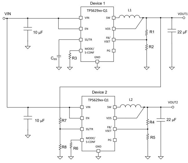
Figure 8-5. Schematic for Ratiometric and Simultaneous Start-Up
