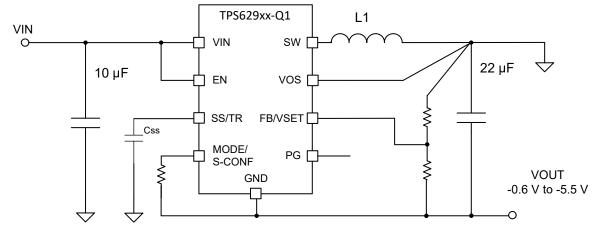
Figure 9-86. IBB Example with Adjustable Feedback
