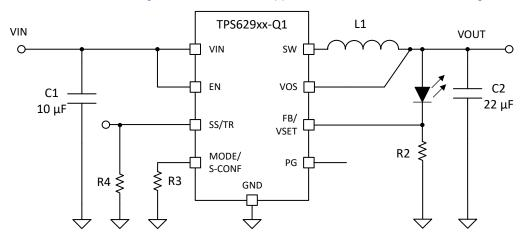
Figure 9-82. Single Power LED Supply
