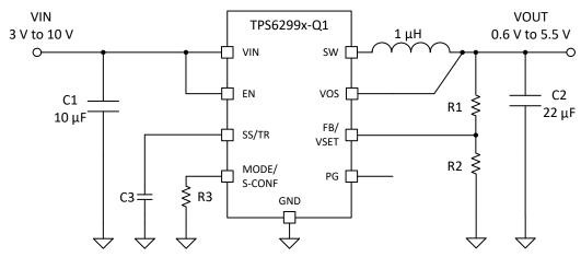
Figure 8-2. Adjustable  $V_{\text{O}}$  Operation Schematic
