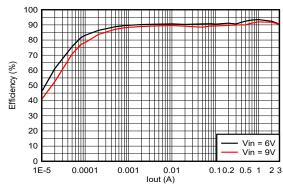
Efficiency Versus Output Current (3.3 Vo at 2.5 MHz, 1 µH, Auto PFM or PWM)
