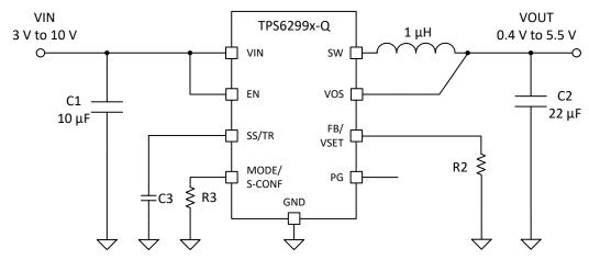
Figure 9-39. Typical Application Circuit (VSET)
