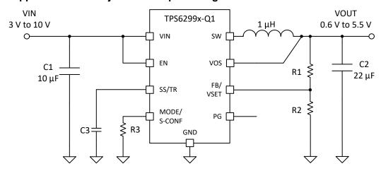
Figure 9-1. Typical Application Circuit
