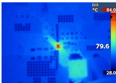
Figure 10-8. Case Temperature, V_{IN} = 24\text{ V} , I_{OUT} = 3\text{ A} , f_{SW} = 500\text{ kHz}
