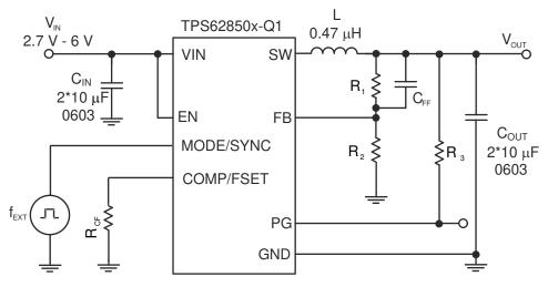
Figure 9-58. Schematic using External Synchronization
