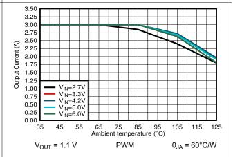
Figure 9-18. Output Current vs Ambient Temperature
