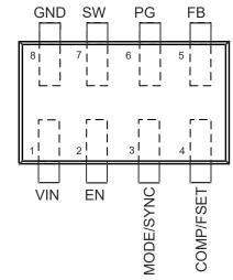
Figure 5-1. 8-Pin SOT583 DRL Package for TPS62850x-Q1 (Top View)
