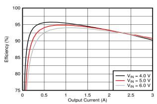
Efficiency vs  $I_{OUT}$ ,  $V_{OUT} = 3.3V$
