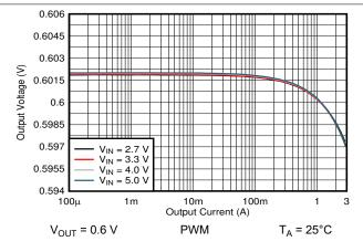
Figure 9-16. Output Voltage vs Output Current
