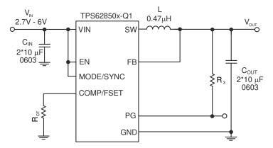
Figure 9-57. Schematic for Fixed Output Voltage Versions
