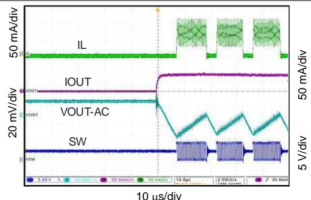
$V(IN) = 4.0\text{ V}$  from bench power supply + additional  $CIN = 100\ \mu\text{F}$
