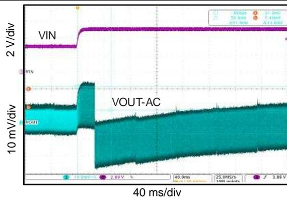
$V(IN) = 3.0\text{ V} \rightarrow 5.0\text{ V}$  from bench power supply
