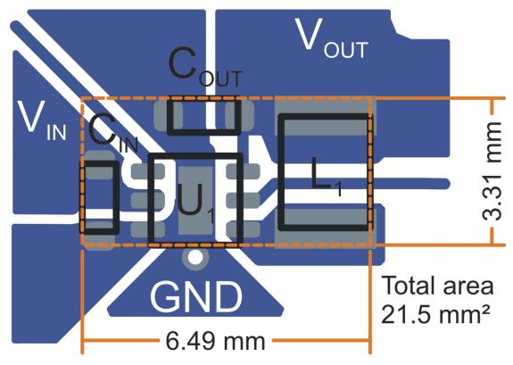
Figure 33. Suggested Layout for Fixed-Output-Voltage Options
