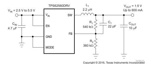
Figure 31. TPS62560 Adjustable 1.5-V Output
