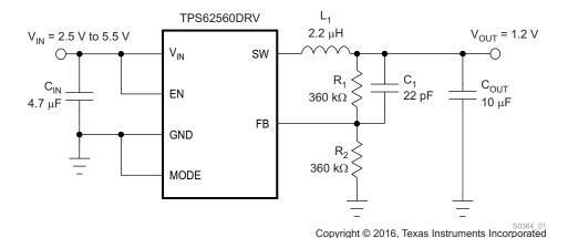
Figure 30. TPS62560 Adjustable 1.2-V Output
