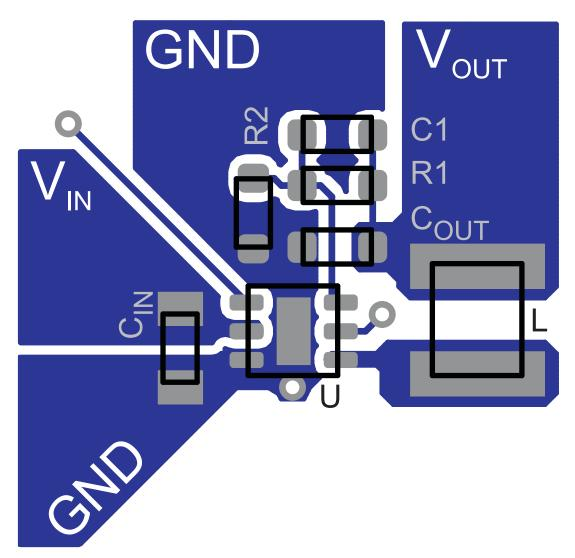
Figure 34. Suggested Layout for Adjustable-Output-Voltage Version
