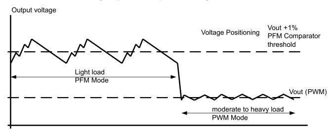
Figure 5. Power Save Mode Operation With Automatic Mode Transition
