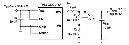
Figure 21. TPS62290DRV Adjustable 3.3 V
