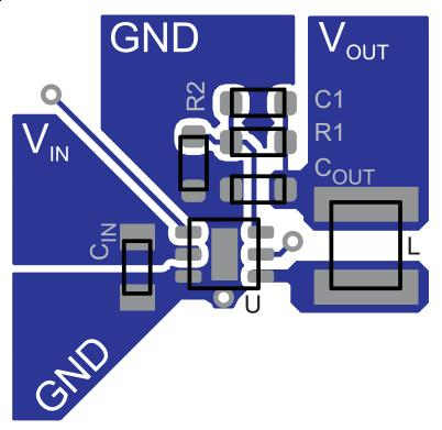
Figure 24. Layout Diagram
