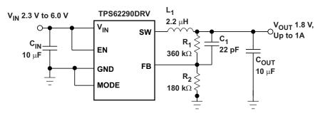
Figure 6. TPS62290DRV Adjustable 1.8 V
