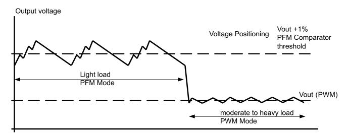
Figure 5. Power Save Mode Operation
