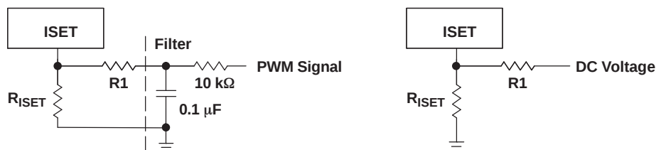
Figure 10. Analog Dimming Using an External Voltage Source to Control the Output Current
