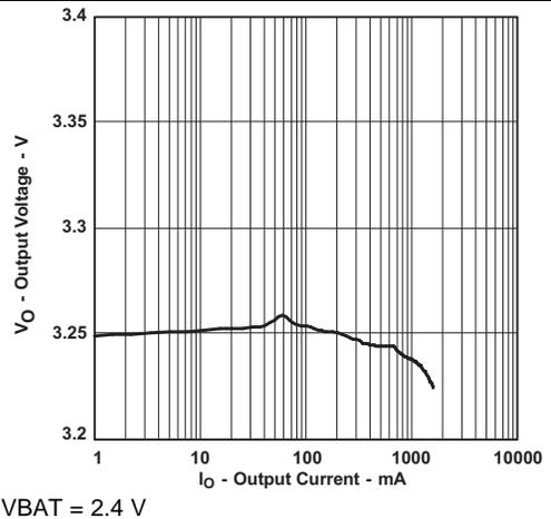
Figure 8. TPS61031 Output Voltage vs Output Current
