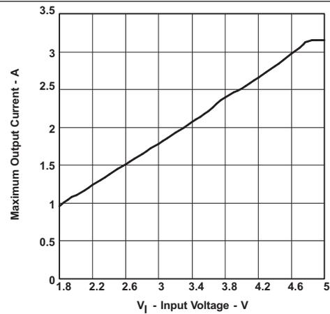
**Figure 2. TPS61032 Maximum Output Current vs Input Voltage**
