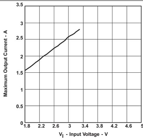
**Figure 1. TPS61031 Maximum Output Current vs Input Voltage**
