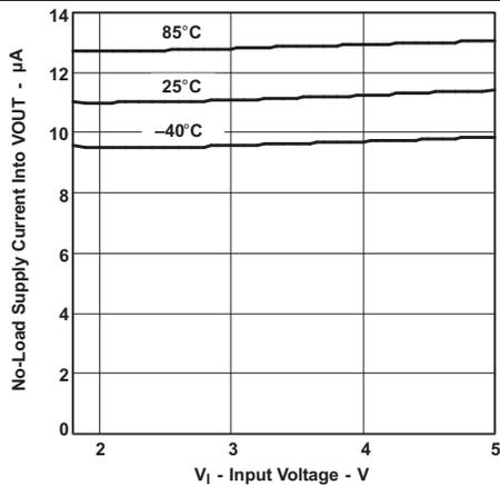
Figure 11. TPS61032 No-Load Supply Current Into Vout vs Input Voltage
