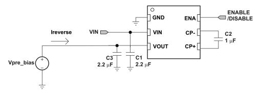
Figure 5. Output Reverse Current Test Setup
