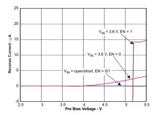
Figure 6. Reverse Current Test Results (Typical)
