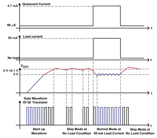
Figure 7. Normal Mode and Skip Mode Operation
