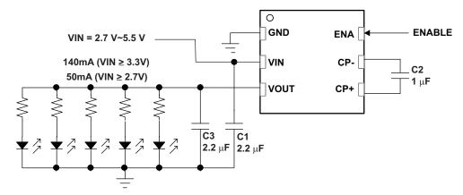
Figure 26. Application Circuit for Driving White LEDs
