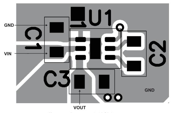
Figure 27. Recommended PCB Layout
