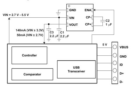
Figure 10. Application Circuit for OTG System
