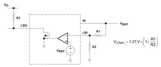
Figure 5. Programming of the Low-Battery Comparator Trip Voltage
