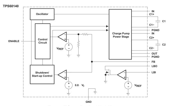
Figure 3. TPS60140 Functional Block Diagram
