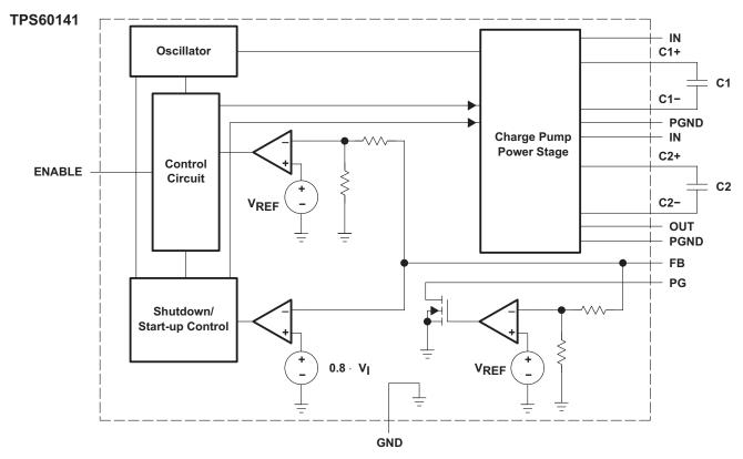
Figure 4. TPS60141 Functional Block Diagram
