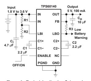
Figure 6. Typical Application Schematic
