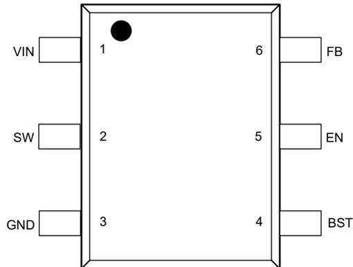
**Figure 4-1. 6-Pin SOT563 DRL Package (Top View)**
