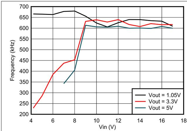
Figure 5-7. Frequency vs Input Voltage at 2A Loading
