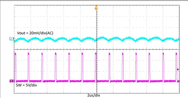
**Figure 7-9. TPS562206 Output Voltage Ripple With 0.1A Loading**
