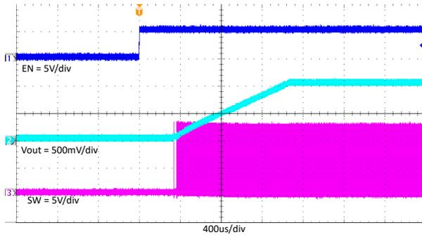
**Figure 7-14. TPS562206 Enable On With 2A Loading**
