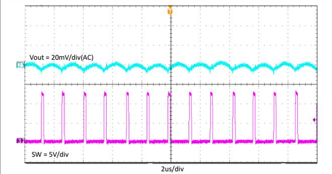
**Figure 7-11. TPS562206 Output Voltage Ripple With 2A Loading**
