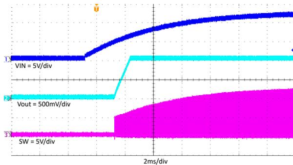
**Figure 7-18. TPS562206 Power On With 2A Loading**
