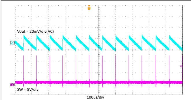
**Figure 7-8. TPS562203 Output Voltage Ripple With 0.1A Loading**
