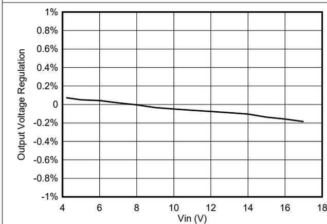
Figure 7-6. TPS562203 Line Regulation vs Vin at 1A Loading
