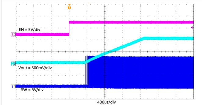
**Figure 7-12. TPS562203 Enable On With 2A Loading**
