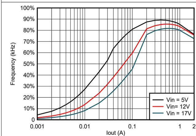
Figure 5-11. TPS562206 Efficiency at 0.6 Vout With 1.5uH Inductor
