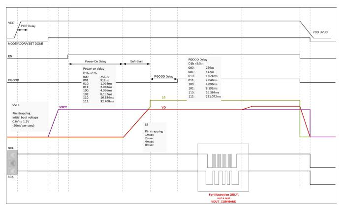
Figure 31. Startup and VOUT\_COMMAND Timing Diagram
