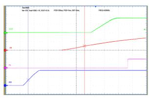
Figure 27. Proper Sequencing of  $V_{DD}$  and  $EN\_UVLO$  to Support the Use of 4-ms SS Setting
