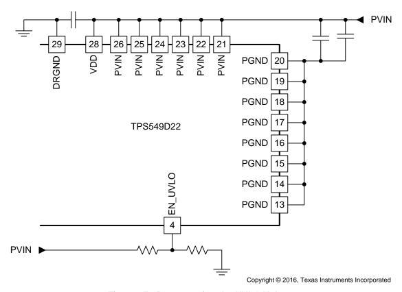
Figure 25. Programming the UVLO Voltage
