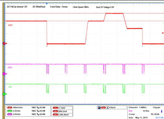
Figure 13. PMBus 1-MHz Bus Speed with 1.8-V Pullup
