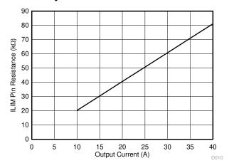
Figure 6-4. Current Limit Resistance vs OCP Valley Overcurrent Limit
