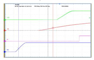
Figure 6-5. Proper Sequencing of V<sub>DD</sub> and EN\_UVLO to Support the use of 4-ms SS Setting
