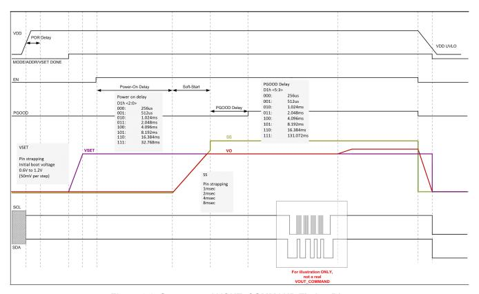
Figure 6-9. Start-up and VOUT\_COMMAND Timing Diagram
