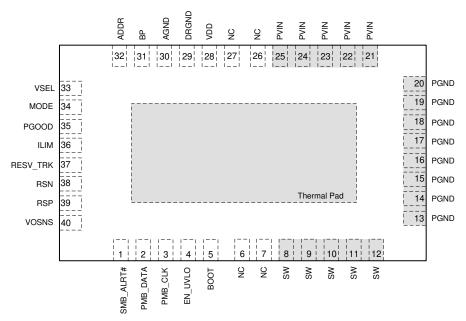
Figure 4-1. RVF Package 40-Pin LQFN-CLIP With Thermal Pad Top View
