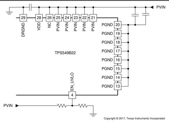
Figure 6-3. Programming the UVLO Voltage
