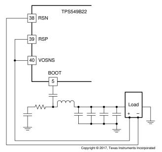
Figure 6-7. Remote Sensing Without Feedback Resistors
