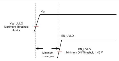
Figure 6-6. Minimum Delay Between V<sub>DD</sub> and EN\_UVLO to Support the use of 4-ms and 8-ms SS settings
