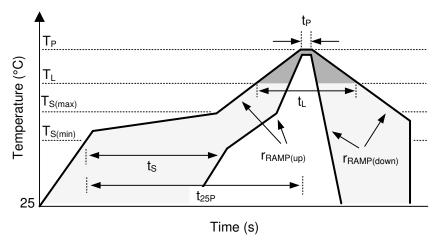
Figure 8-16. Recommended Reflow Oven Thermal Profile
