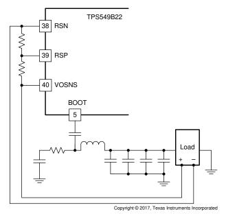
Figure 6-8. Remote Sensing With Feedback Resistors
