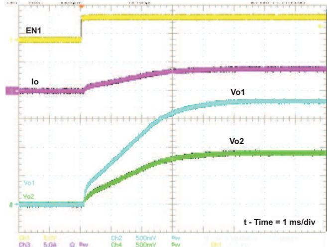
Figure 26. Ratio-metric Startup
