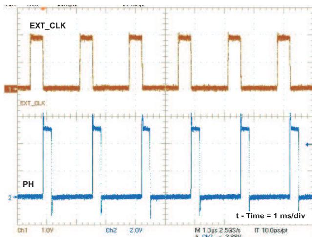
Figure 29. Synchronizing to a System Clock
