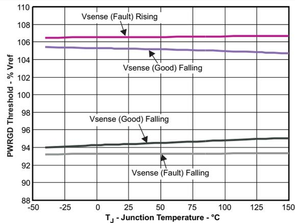
Figure 15. PWRGD Threshold vs Temperature
