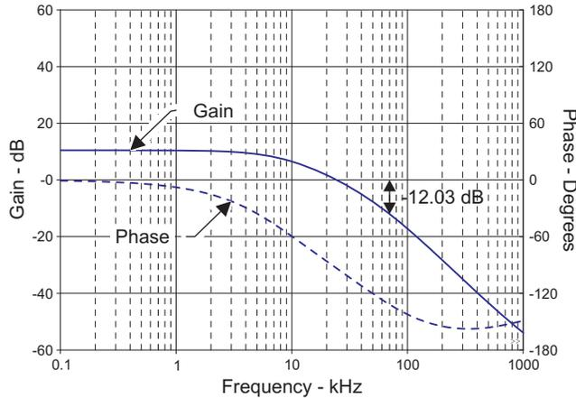
**Figure 37. Power Stage Gain and Phase Characteristics**
