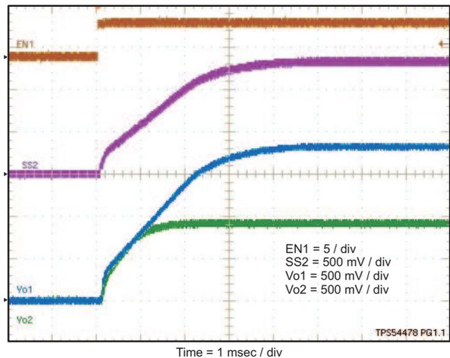
**Figure 28. Simultaneous Start-Up using Coupled SS/TR Pins**
