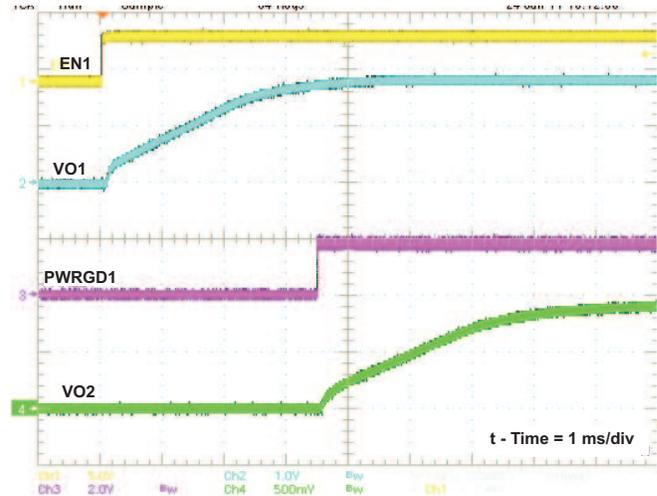
Figure 24. Sequential Startup using EN and PWRGD
